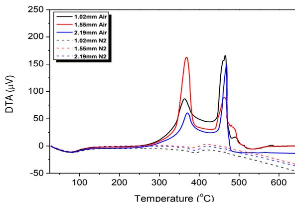
Figure 3. DTA curve of pine sawdust *in natura* in different particle sizes and atmospheres
