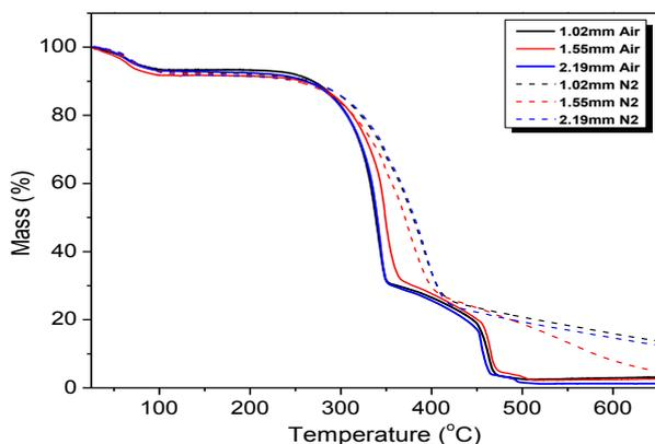
Figure 1. TG curve of pine sawdust *in natura* in different particle sizes and atmospheres
