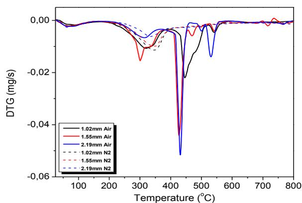
Figure 11. DTG curve of coffee husks torrefied in different particle sizes and atmospheres
