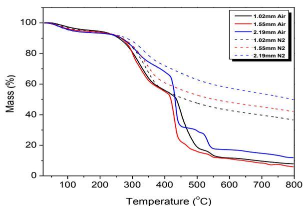
Figure 10. TG curve of coffee husks torrefied in different particle sizes and atmospheres
