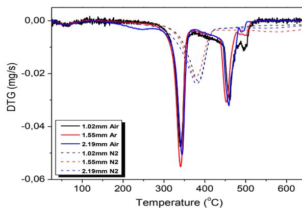
Figure 4. TG curve of torrefied pine sawdust in different particle sizes and atmospheres
