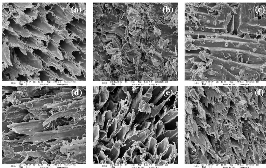
Figure 13. Images SEM pine sawdust *in natura*: (a) 2.19 mm; (b) 1.55 mm; (c) 1.02 mm and torrefied: (d) 2.19 mm; (e) 1.55 mm; (f) 1.02 mm
