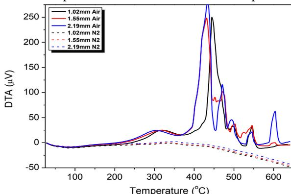
Figure 12. DTA curve of coffee husks torrefied in different particle sizes and atmospheres
