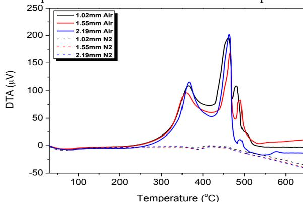
Figure 5. DTG curve of torrefied pine sawdust in different particle sizes and atmospheres
