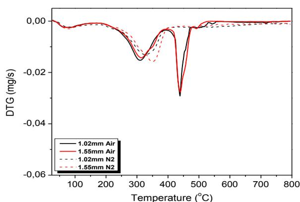
Figure 7. TG curve of coffee husks *in natura* in different particle sizes and atmospheres
