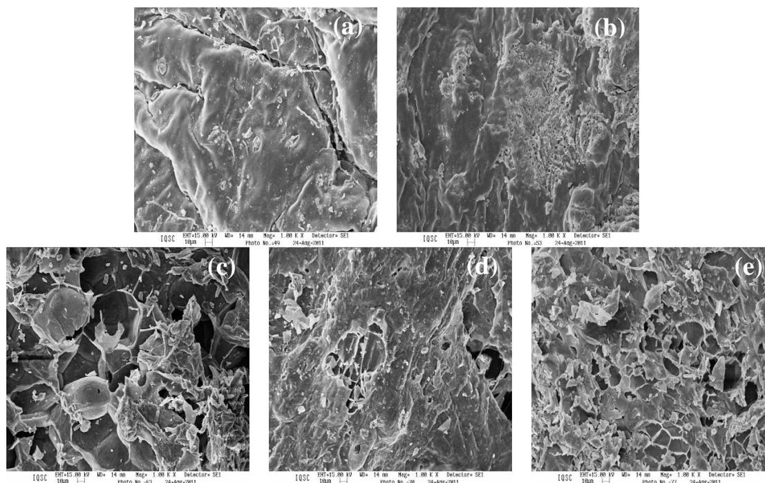
Figure 14. Images SEM coffee husks *in natura*: (a) 1.55 mm; (b) 1.02 mm and torrefied: (c) 2.19 mm; (d) 1.55 mm; (e) 1.02 mm
