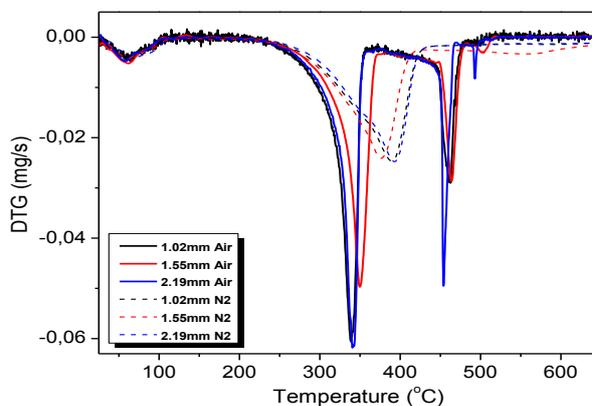
Figure 2. DTG curve of pine sawdust *in natura* in different particle sizes and atmospheres
