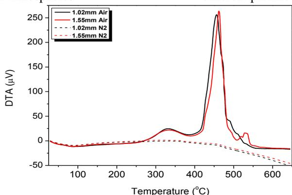
Figure 9. DTA curve of coffee husks *in natura* in different particle sizes and atmospheres
