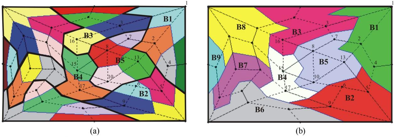
Figure 1. Unstructured mesh: (a) fine mesh divided in blocks, (b) coarse mesh.
