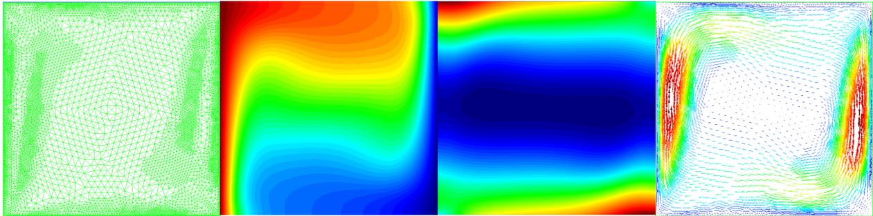
Figure 3: Adaptive mesh, temperature field, pressure field and velocity field for  $Ra = 10^5$  and  $Pr = 0.71$
