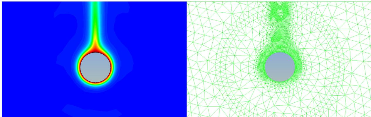
Figure1: Temperature field and final adaptive mesh at  $t = 70d/u_0$  for  $Ra = 5 \times 10^4$  and  $Pr = 0.71$
