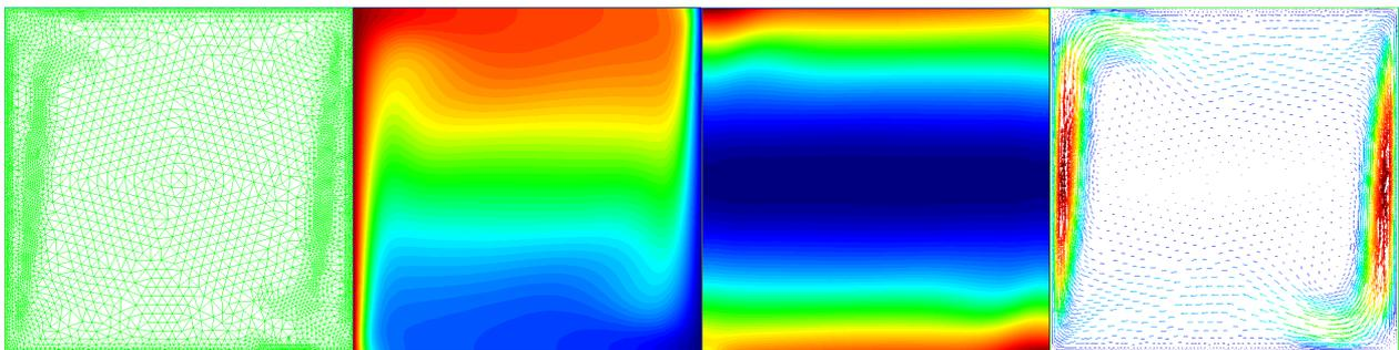
Figure 4: Adaptive mesh, temperature field, pressure field and velocity field for  $Ra = 10^6$  and  $Pr = 0.71$
