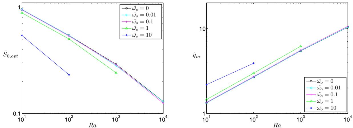
Figure 2: Single scale results for a row of rotating cylinders shown in Fig. 1 for  $Pr = 0.72$ . (Left: Optimal cylinder-to-cylinder spacings; Right: Maximum heat transfer density rates)
