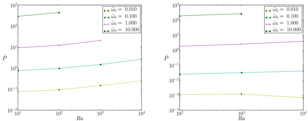
Figure 4: Non-dimensional power input required to rotate the cylinders shown in Fig. 1 for  $Pr = 0.72$ . (Left: Single scale configuration; Right: Multi scale configuration)
