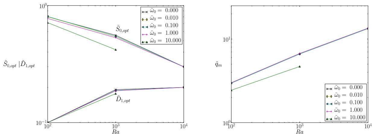
Figure 3: Multi scale results for a row of rotating cylinders shown in Fig. 1 for  $Pr = 0.72$ . (Left: Optimal cylinder packing; Right: Maximum heat transfer density rates)
