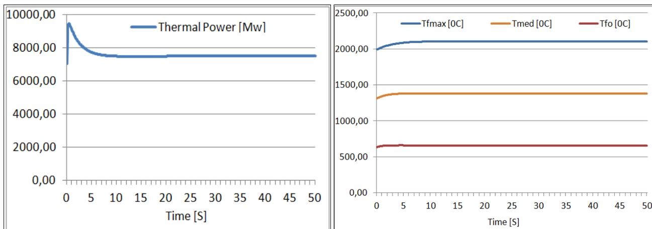
Figure 3. Behavior of Thermal Power and Temperature fields during the first 50 seconds of the transient.
