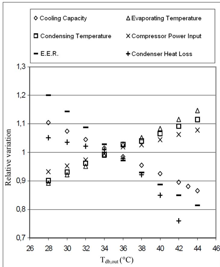
Figure 7. Variation of characteristics as function of outdoor dry-bulb temperature ( $T_{db,out}=35.0^{\circ}\text{C}$ ,  $T_{db,in}=26.7^{\circ}\text{C}$ ).
