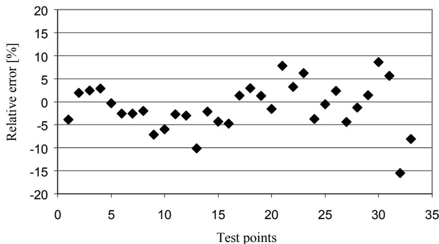
Figure 3. Condenser heat transfer rate relative errors.
