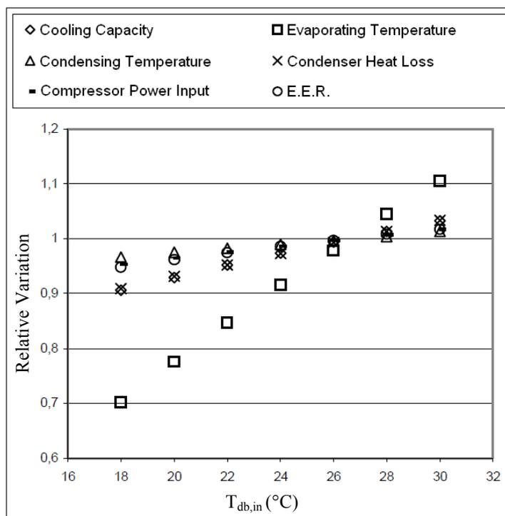
Figure 6. Variation of characteristics as function of indoor dry-bulb temperature ( $W_{out}=0,010\text{kg/kg}$ ,  $T_{db,out}= 35^{\circ}\text{C}$ ).
