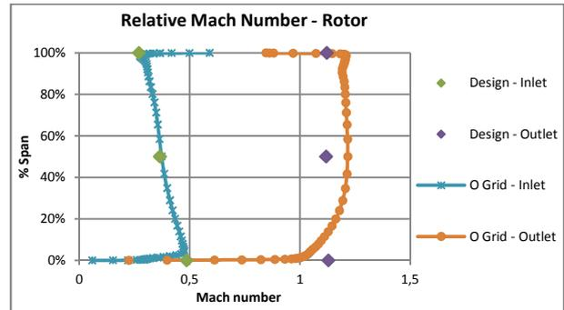
Figure 8. Mach Distribution – Rotor
