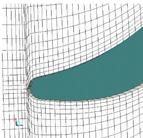
Figure 4. H-grid generated in a turbine blade
