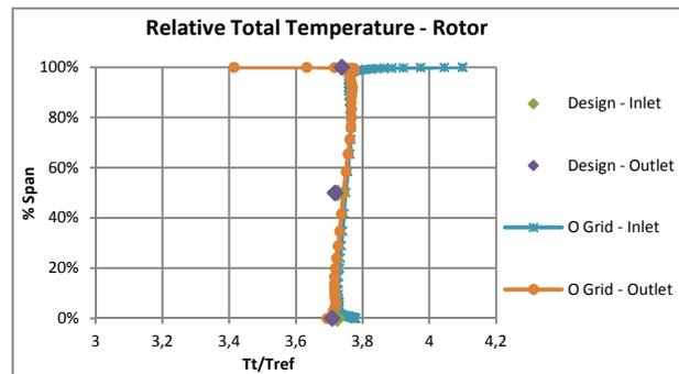
Figure 12. Temperature Distribution – Rotor
