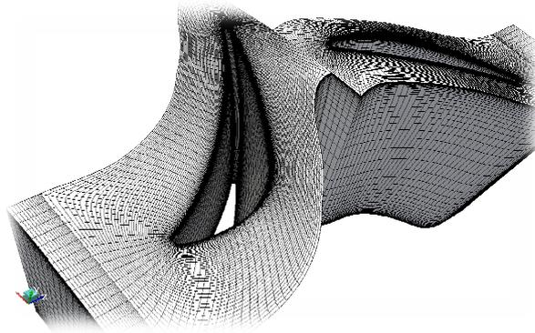
Figure 6. O-grid generated for a single-stage axial turbine
