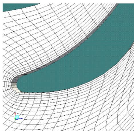
Figure 5. O-grid generated in a turbine blade
