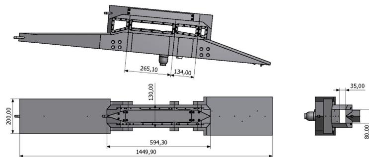
Figure 6. The truncated 14-X waverider scramjet model main dimensions.
