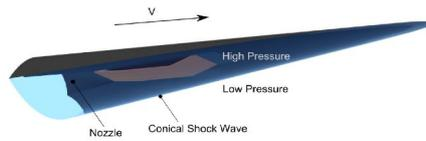
Figure 2. Hypersonic waverider vehicle concept.
