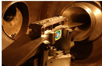
Figure 7. Instrumented truncated 14-X waverider scramjet model installed at the T3 Hypersonic Shock Tunnel.
