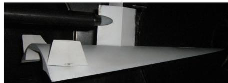
Figure 4. Instrumented “waverider” model installed at T3 Hypersonic Shock Tunnel.
