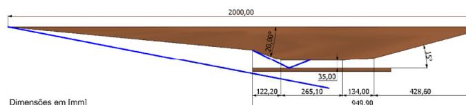
Figure 5. The 14-X waverider scramjet Mach number 10 model main dimensions.
