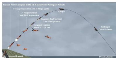
Figure 10. Hypersonic Accelerator Vehicle and 14-X Hypersonic Aerospace Vehicle in ballistic trajectory.
