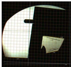
Figure 8. Mach number 7 flow past the model leading edge aligned if the horizontal.
