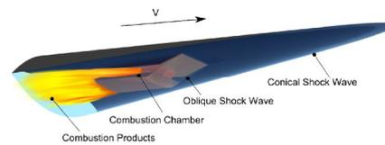
Figure 3. Hypersonic scramjet airbreathing propulsion concept.
