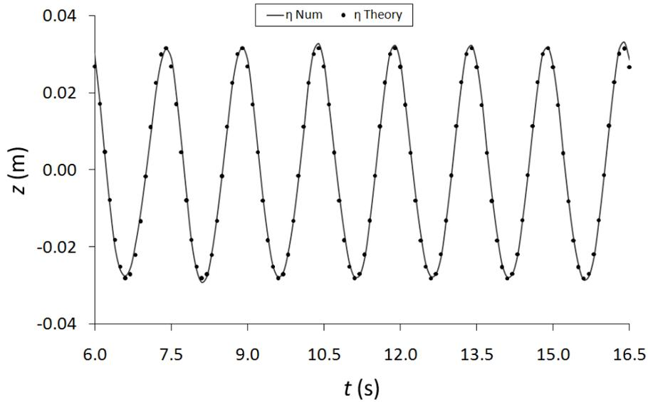
Figure 3. Comparison between numerical model and the second order Stokes theory.
