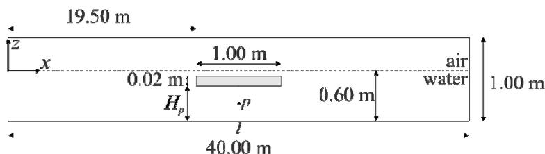
Figure 2. Geometry of the tank and the plate.
