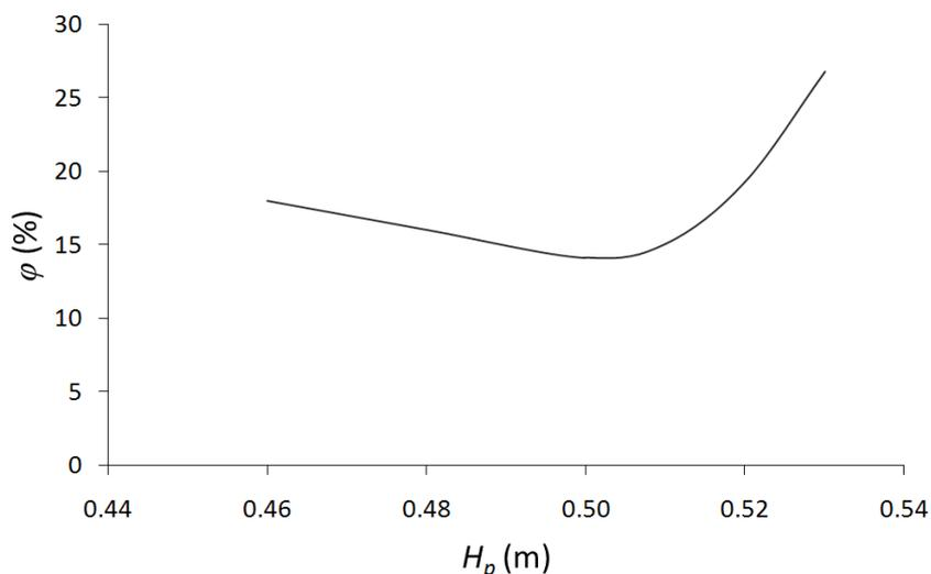
Figure 8. Efficiency of the submerged plate wave energy converter for different plate heights.
