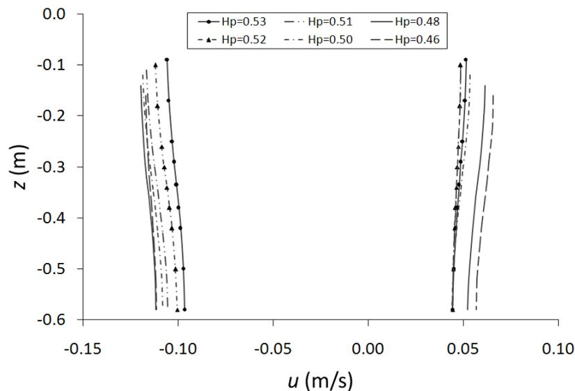
Figure 5. Maximum velocity profiles: the same wave propagation direction and the opposite direction.
