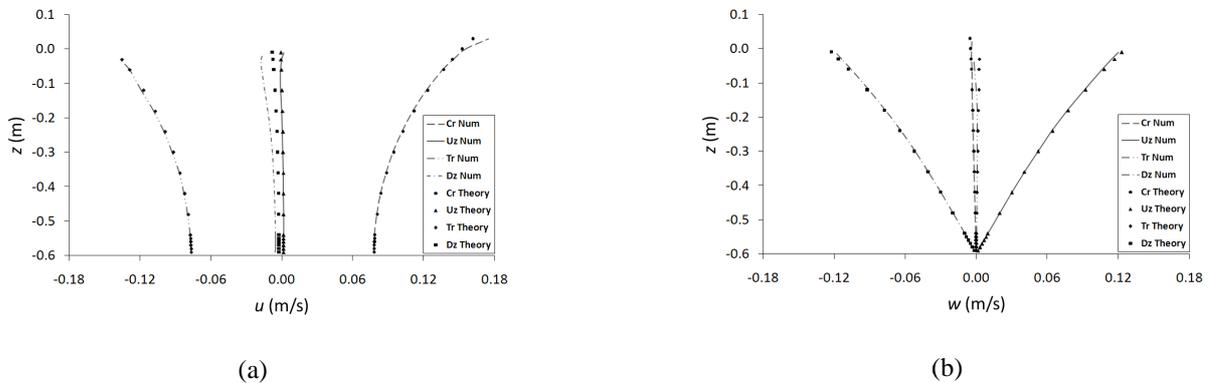
Figure 4. Numerical versus analytical results (second order Stokes theory) for velocity components  $u$  and  $w$ .
