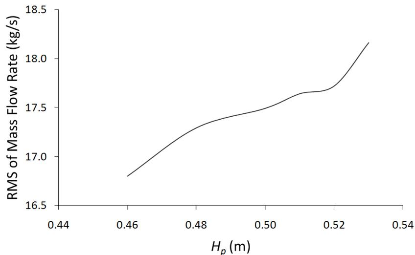
Figure 7. Root mean square (RMS) of the mass flow under the plate for each case.
