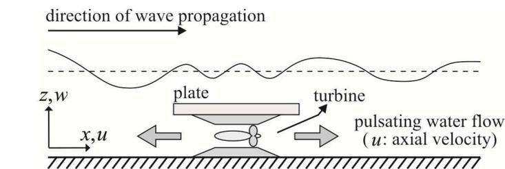
Figure 1. The working principle of the submerged plate type converter.
