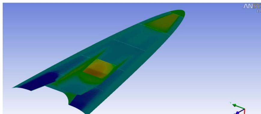
Figure 9: rate heat under vehicle for Mach 6.
