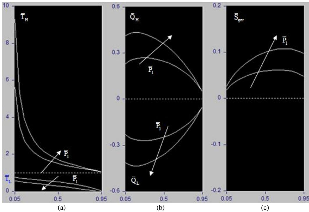
Figure 4. The  $x$  and  $\bar{P}_1$  variation of (a) the hot and cold gas temperatures  $\bar{T}_H$  and  $\bar{T}_L$ , (b) the Vortex Tube potential for heating  $\bar{Q}_H$  or cooling  $\bar{Q}_L$  and (c) the entropy generation  $\bar{S}_{gen}$  ( $\xi = 0.8, \bar{P}_1 = 2, \bar{P}_1 = 5$ ).
