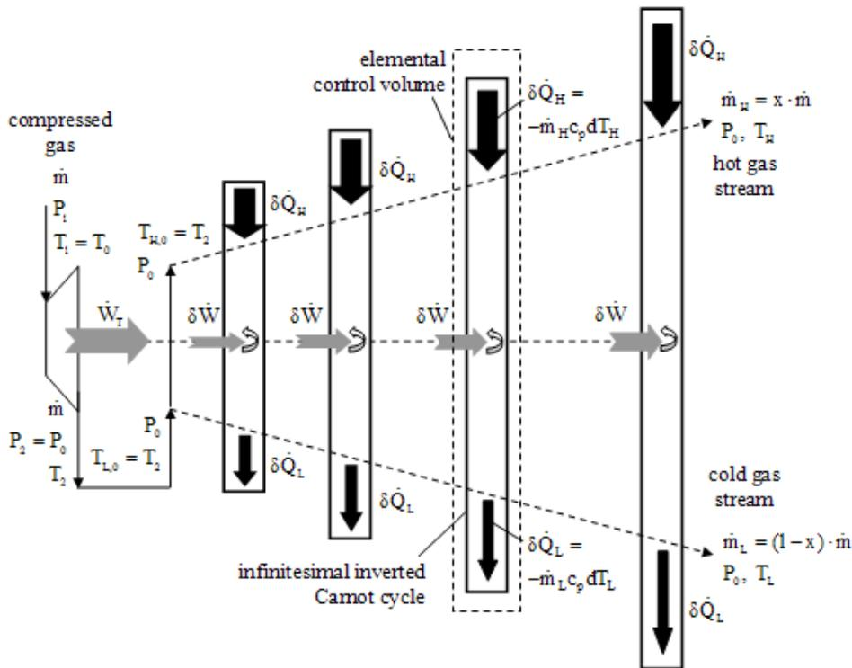
Figure 2. RHVT thermodynamic model based on infinitesimal inverted Carnot cycles.
