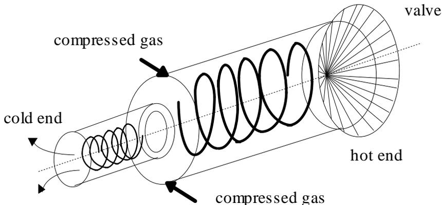
Figure 1. Schematic view of the Ranque-Hilsch Vortex Tube.
