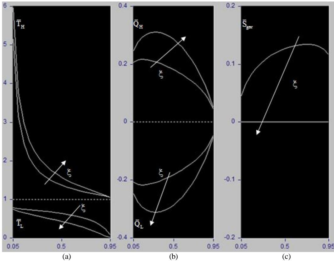
Figure 3. The  $x$  and  $\xi$  variation of (a) the hot and cold gas temperatures  $\bar{T}_H$  and  $\bar{T}_L$ , (b) the Vortex Tube potential for heating  $\bar{Q}_H$  or cooling  $\bar{Q}_L$  and (c) the entropy generation  $\bar{S}_{gen}$  ( $\xi = 1, \xi = 0.5, \bar{P}_1 = 2$ ).
