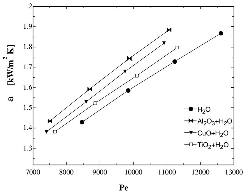
Figure 4. Convective heat transfer coefficient on the shell side,  $j = 2,0\%$   $d_p = 20nm$
