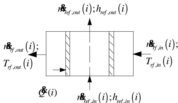
Figure 2. Scheme of the i-th heat exchanger element
