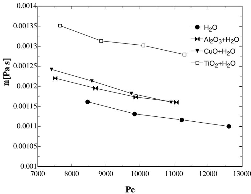
Figure 6. Dynamic viscosity of the cooled fluid flow.  $j = 2,0\%$   $d_p = 20nm$
