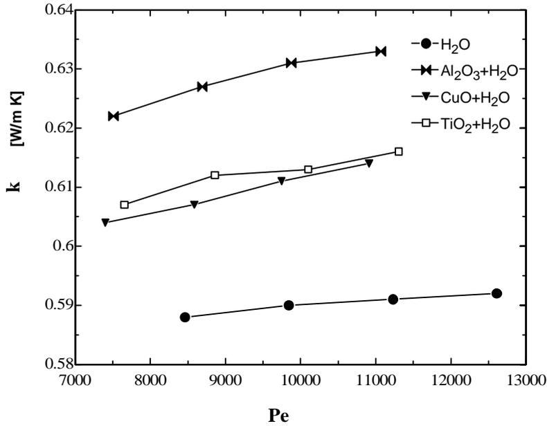
Figure 5. Thermal conductivity of the cooled fluid flow.  $j = 2,0\%$   $d_p = 20nm$
