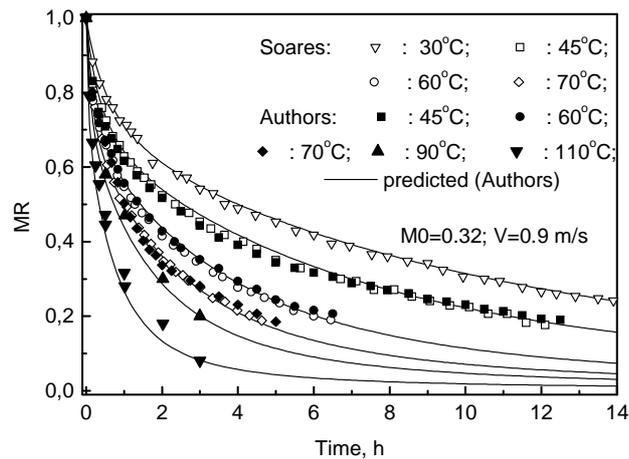
Figure 5. Temperature influence on soybean drying dynamics.
