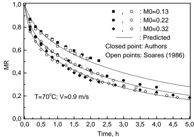
Figure 2. Soybean drying dynamics in a thin-layer at different initial grain moisture contents: T=70°C
