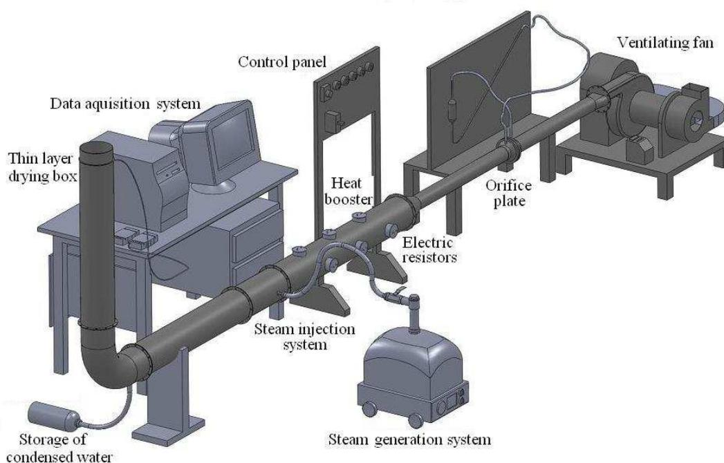
Figure 1. Experimental equipment developed for tests.
