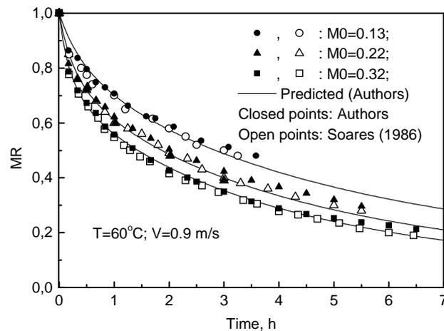
Figure 3. Soybean drying dynamics in a thin-layer at different initial grain moisture contents: T=60°C.
