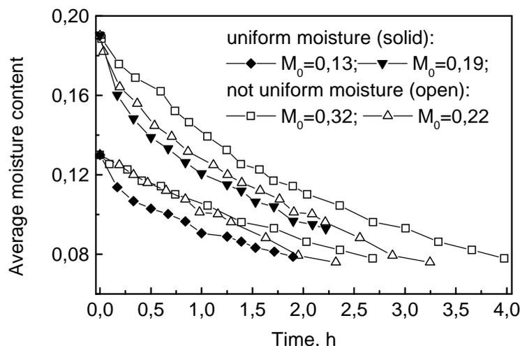
Figure 7. Soybean drying dynamics in thin- layer with "uniform" and "non uniform" initial distribution of moisture inside of grain.
