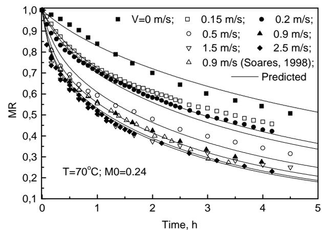
Figure 6. Velocity influence on soybean drying dynamics.
