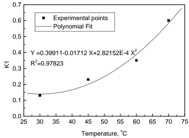
Figure 8. Dependence of coefficient  $k_1$  from drying temperature.
