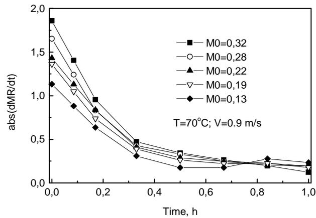
Figure 4. Dynamics of absolute drying rate variation in a thin layer at different initial grain moisture contents
