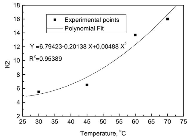
Figure 9. Dependence of coefficient  $k_2$  from drying temperature.
