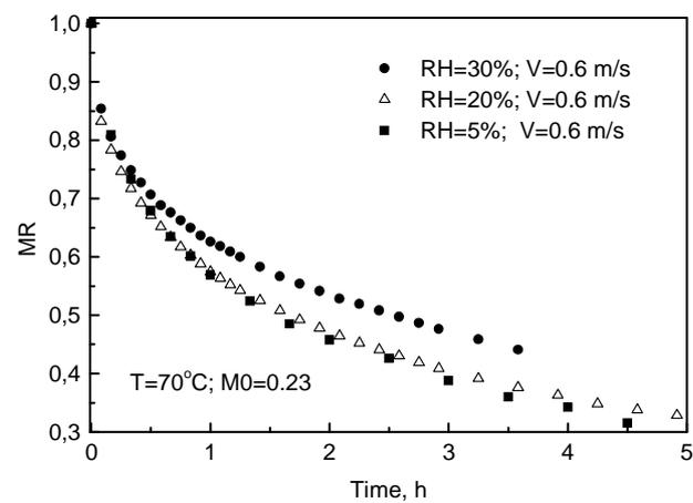
Figure 10. Influence of air relative humidity on thin-layer drying.
