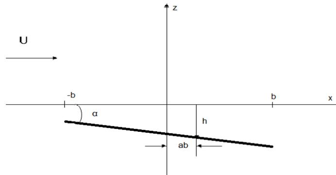
Figure 1. Coordinate system: airfoil in heaving motion and with angle of attack  $\alpha$
