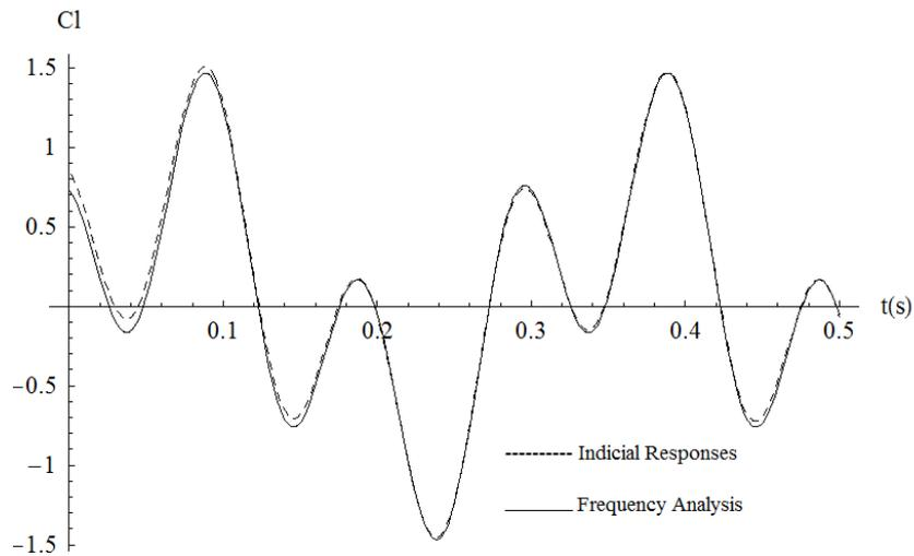
Figure 6. Lift coefficient – superposition of the motions.
