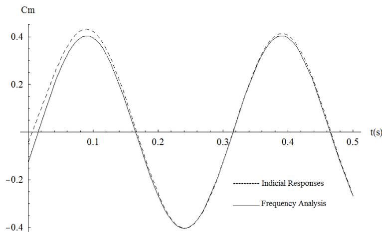
Figure 5. Moment coefficient about the center of the airfoil – pitching movement.
