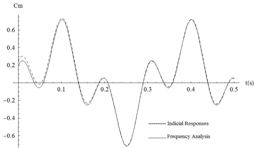
Figure 7. Moment coefficient about the center of the airfoil – superposition of the motions.
