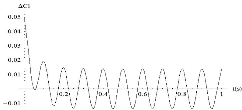
Figure 8. Lift coefficient difference between both methods – heaving motion
