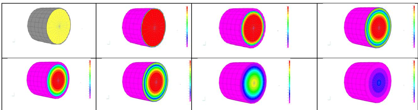
Fig3. FEM model and outputs for the thermal module and sample during the cooling time. The colors represent temperatures. The aluminium cylinder is supposed to be always at the refrigerator temperature ( $10^\circ\text{C}$ ) while the sample temperatures change between  $25^\circ\text{C}$  (red) and  $10^\circ\text{C}$  (pink) as the heat goes from inside to outside (left to right/up to down) .
