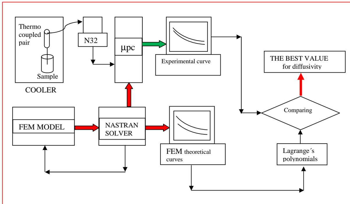
Figure 1: The method strategy: Measurements are compared with theoretical curves until the best values for parameters are achieved
