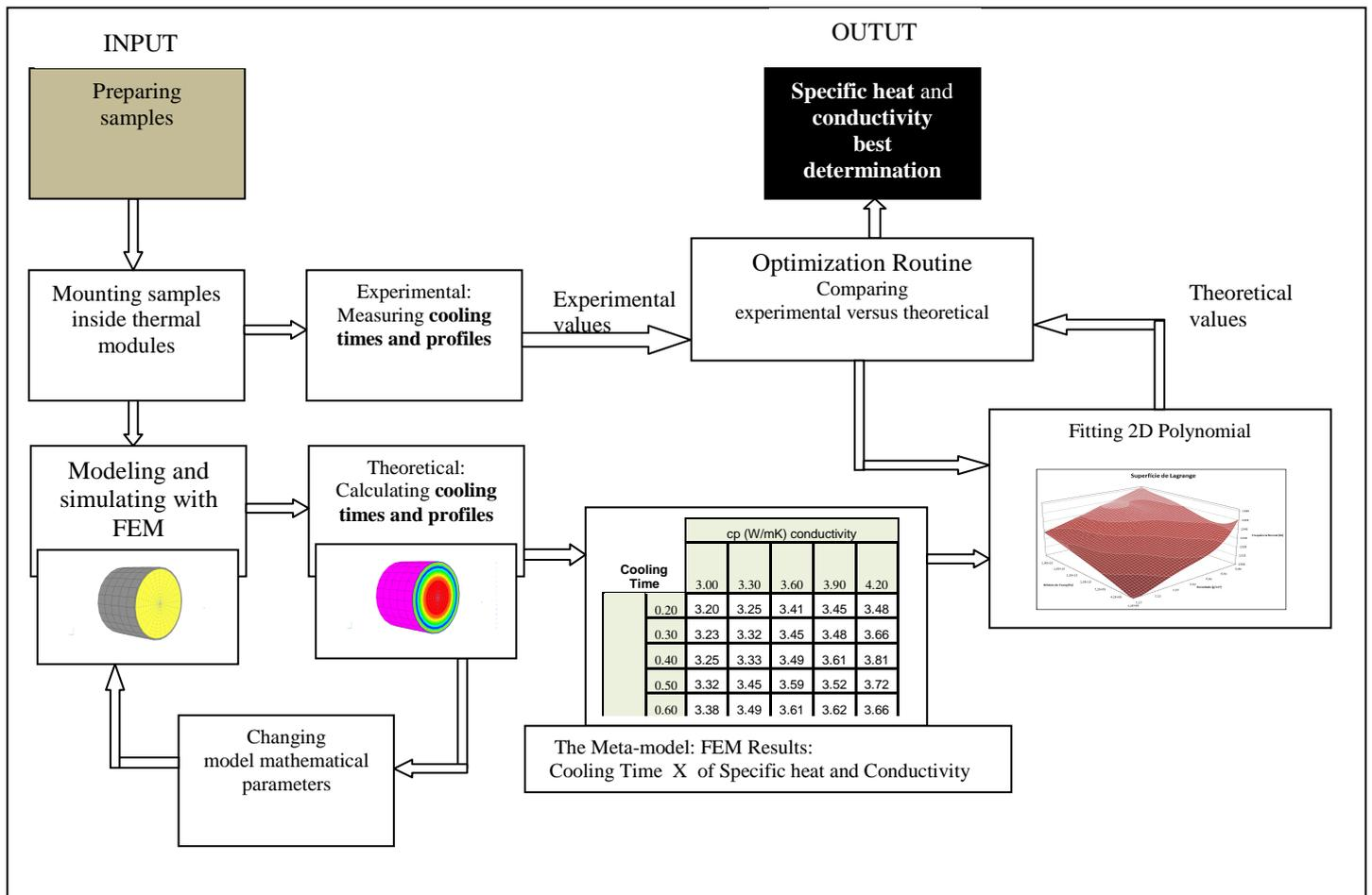
Fig5. The method strategy: Measurements are compared with theoretical curves until the best values for thermo physical parameters are achieved
