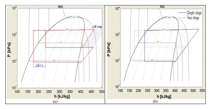
**Figure 6:** Two-stage P-h diagram from figure 5 system (a) and corresponding theoretical single stage P-h diagram operating with the same suction and discharge pressures (b)
