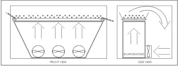
Figure 3: Schematic of a fluidized bed freezer
