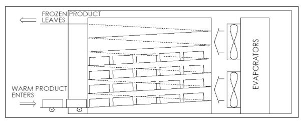
Figure 2: Schematic of a typical spiral Belt freezer
