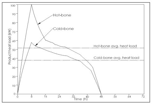
Figure 7: Product heat load characteristics for hot-boned and cold-boned beef cartons [47]
