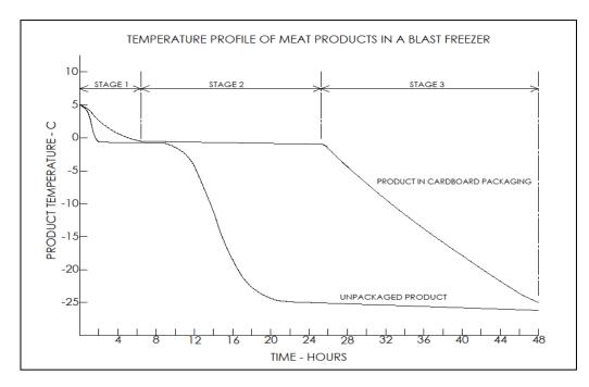
Figure 4: Freezing curves for packaged and unpackaged meat product in an air blast freezer
