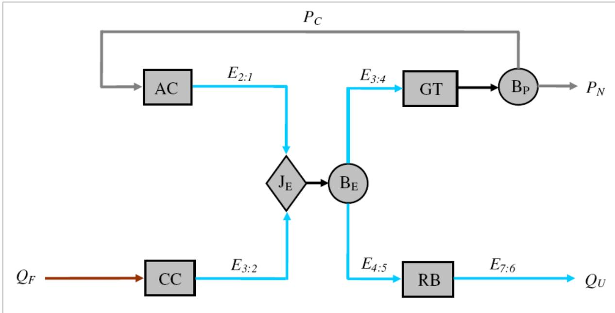
Figure 2. Productive Structure of the Gas Turbine Cogeneration System at Disaggregation Level I
