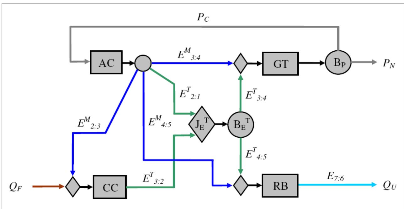
Figure 3. Productive Structure of the Gas Turbine Cogeneration System at Disaggregation Level IIa
