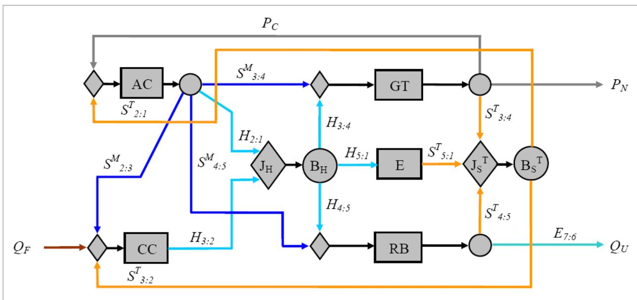
Figure 5. Productive Structure of the Gas Turbine Cogeneration System at Disaggregation Level III
