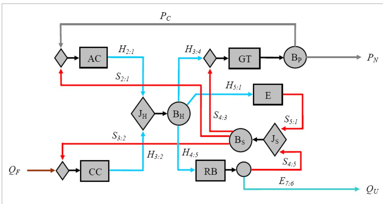
Figure 4. Productive Structure of the Gas Turbine Cogeneration System at Disaggregation Level IIb
