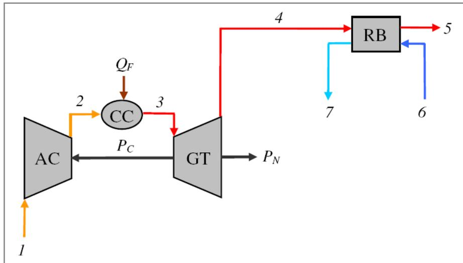
Figure 1. Physical Structure of the Gas Turbine Cogeneration System
