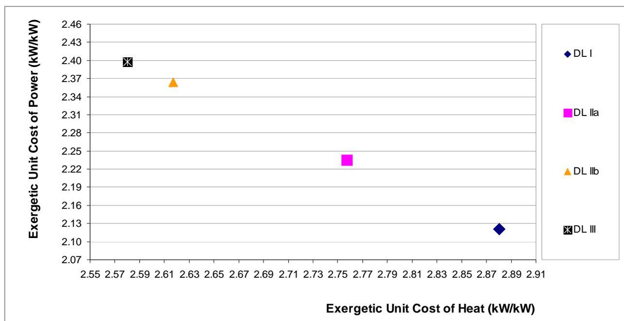
Figure 6. Exergetic Unit Cost of Heat and Power obtained by using Different Disaggregation Levels
