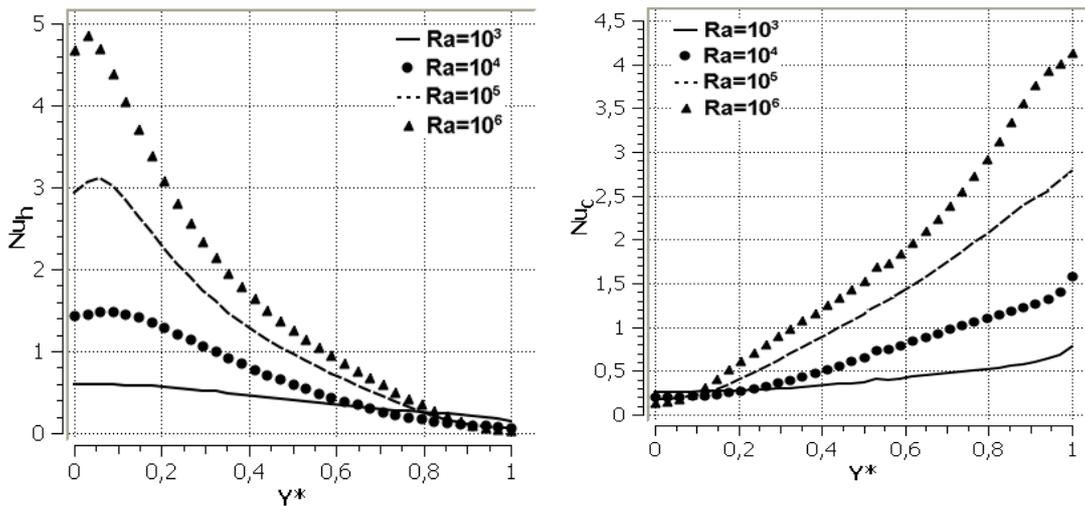
Figure 10. Local Nusselt number for  $Pr = 10$  and  $H_{b1} = H_{b2} = H^*$  in (a) hot and (b) cold wall.
