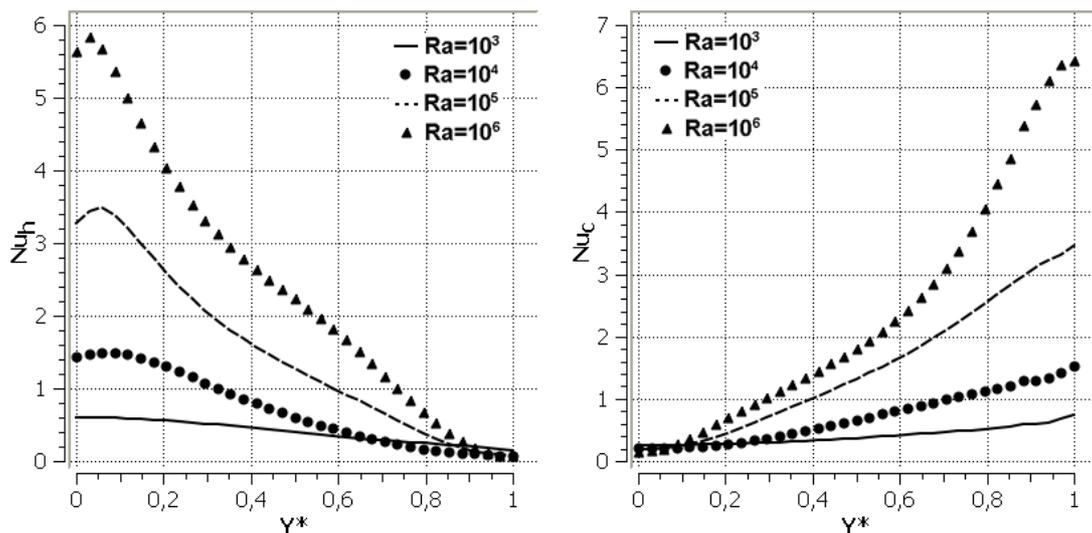
Figure 9. Local Nusselt number for  $Pr = 10$  and  $H_{b1} = H_{b2} = 2H^*/3$  in (a) hot and (b) cold wall.
