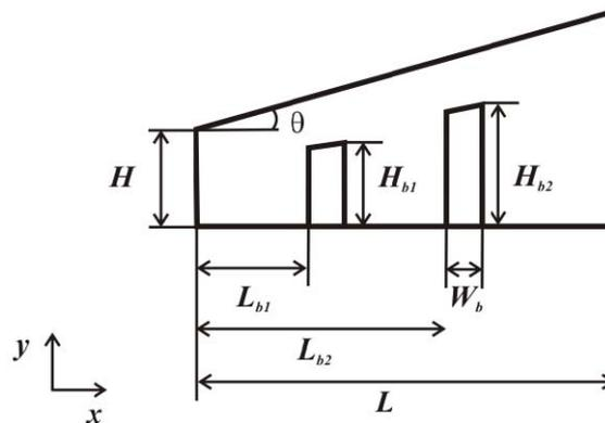
Figure 1. Computational domain for two baffles.
