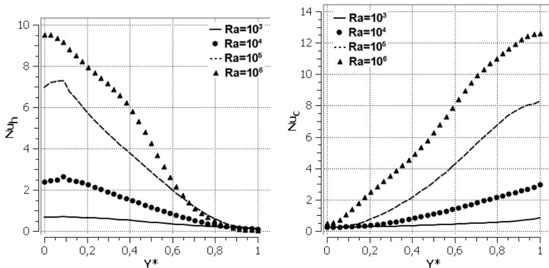
Figure 8. Local Nusselt number for  $Pr = 10$  and  $H_{b1} = H_{b2} = H^*/3$  in (a) hot and (b) cold wall.
