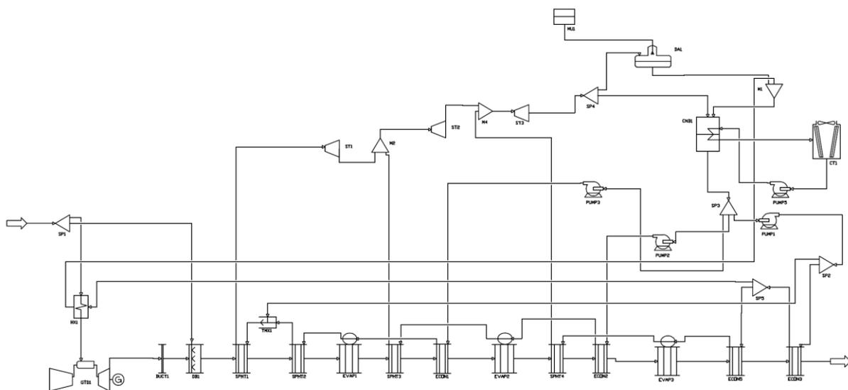
Figure 4. NGCC power plant scheme modeled on GateCycle software
