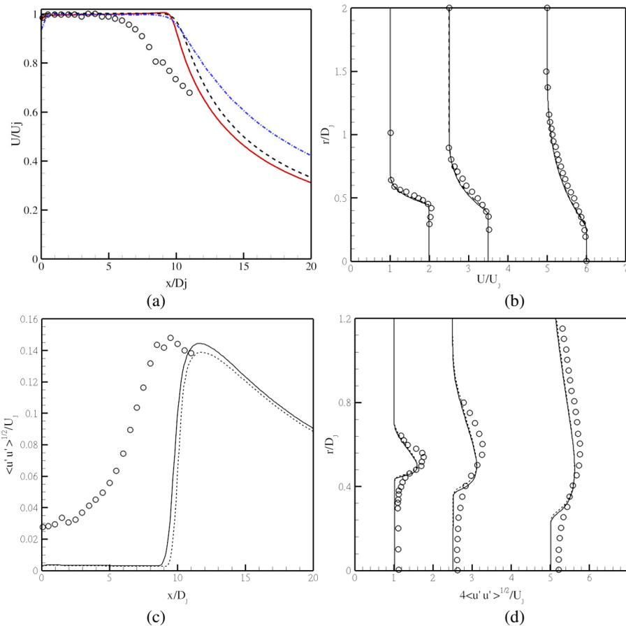
Figure 9. (a) Centerline velocity distribution; (b) Radial profiles of axial velocity; (c) Centerline  $\langle u'u' \rangle^{1/2}/U_j$  distribution; (d) Radial profiles of  $\langle u'u' \rangle^{1/2}/U_j$  at the axial positions  $x/D_j = 1.0$ ,  $x/D_j = 2.5$  and  $x/D_j = 5.0$ : '—' corresponds to 2D axisymmetric result, '- -' corresponds to 3D result, '- · - ·' corresponds to ALMEIDA [2] result and 'o' to experimental results.
