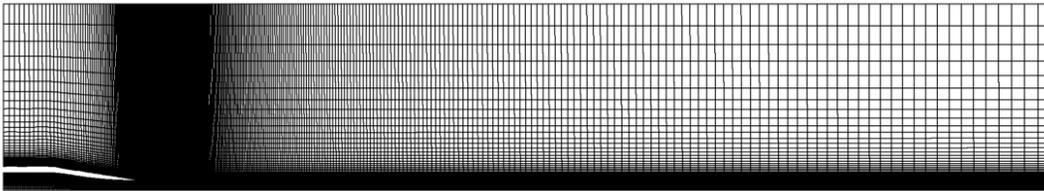
Figure 5. Mesh refinement – axisymmetric domain.
