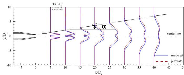
Figure 12 - Turbulent Kinetic Energy Profiles vs  $y$  coordinate along the  $x$  direction.
