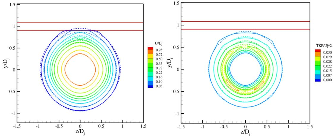
Figure 17. Isovalues of  $U/U_j$ , left, and isovalues of TKE, right, at the plane  $zy$  across the flat plate. The red parallel lines indicate the presence of the plate. (—) Solid line: jet vs plate; (---) Single jet.
