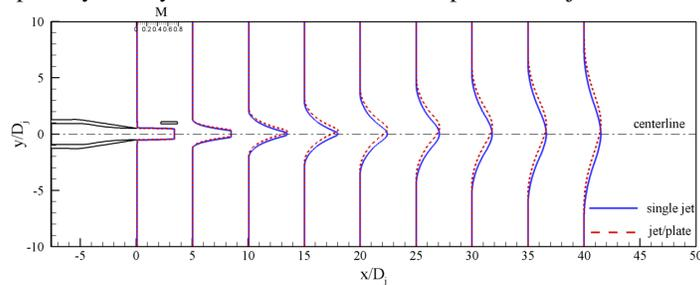
Figure 11 - Mach number profiles vs.  $y$  coordinate along the  $x$  direction.
