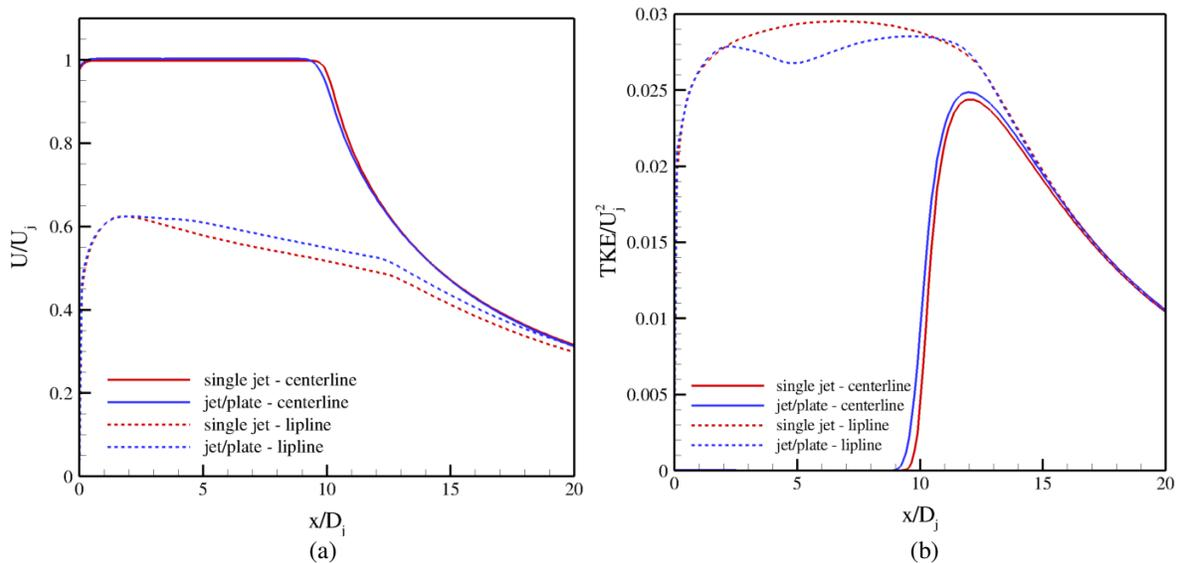
Figure 19 - Axial velocity (a) and TKE (b) distributions at centerline and lipline. Comparison with the 3D single jet – baseline.
