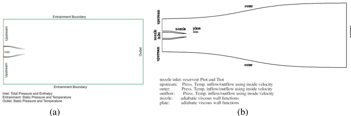
Figure 4. Boundary conditions – (a) Planar Jet Flow; (b) Full 3D domain.
