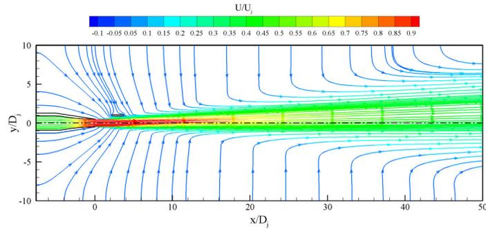
Figure 10. Jet entrainment – Single Jet with Flat Plate.
