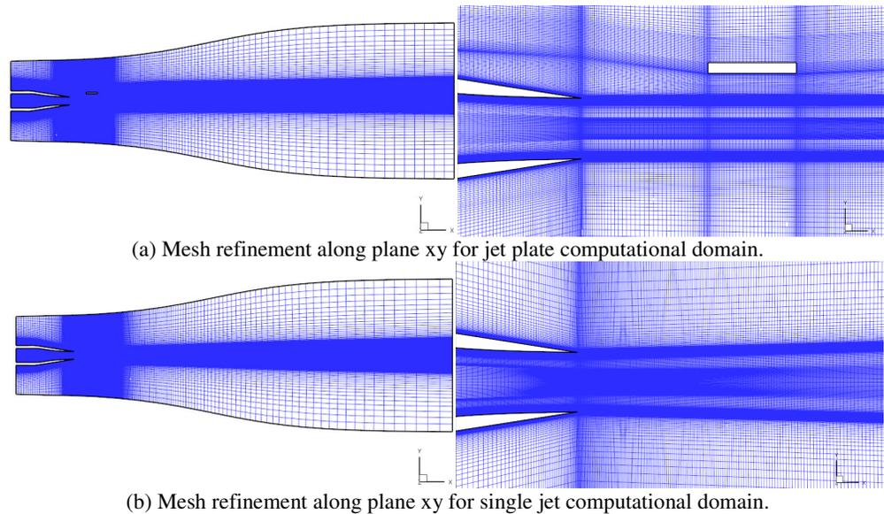
Figure 7. Mesh refinement – (a) jet/plate; (b) single jet - *baseline*.
