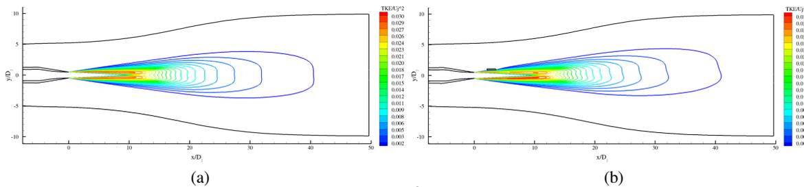
Figure 14 - Snapshot of isovalues of  $TKE/U_j^2$  for: (a) single jet; (b) jet-plate interaction.
