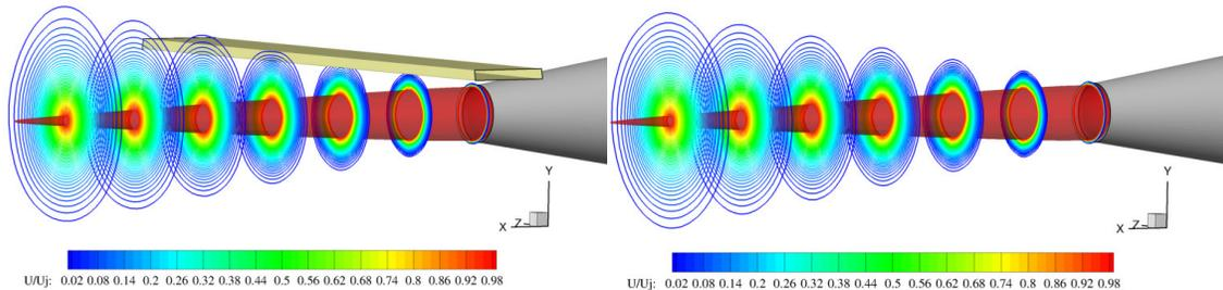
Figure 15. Axial velocity field at planes extracted along axis direction near jet-exit/plate region.
