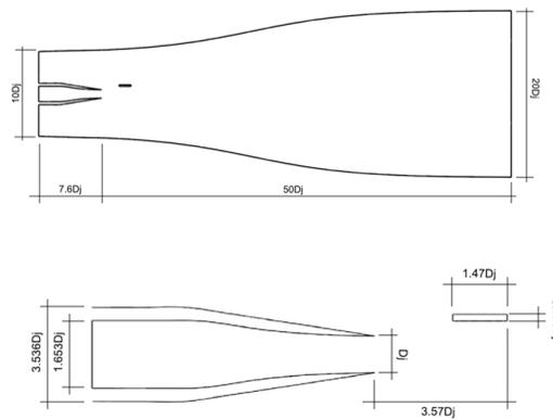
Figure 3. Extend of the computational domain based on jet diameter ( $D_j$ ) – 3D jet flow.
