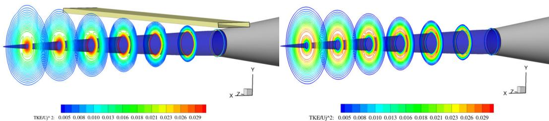
Figure 16. TKE field at planes extracted along axis direction near jet-exit/plate.
