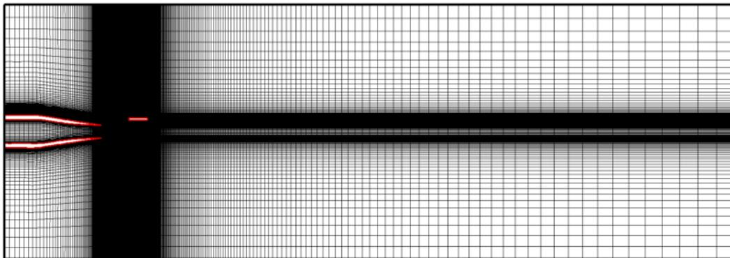
Figure 6. 2D planar domain with flat plate.
