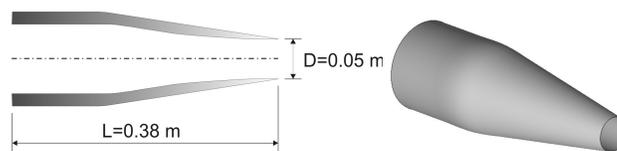
Figure 1. Nozzle geometry for single jet flow.
