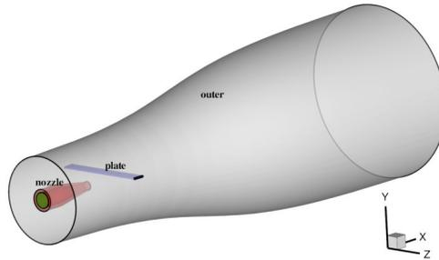
Figure 2. Schematic view of the 3D computational domain for single jet and jet plate interaction RANS simulations.
