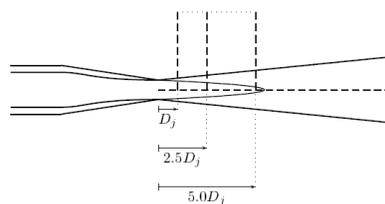
Figure 8. Profiles of axial velocity and second-order moments are obtained along the centerline and along three radial lines.
