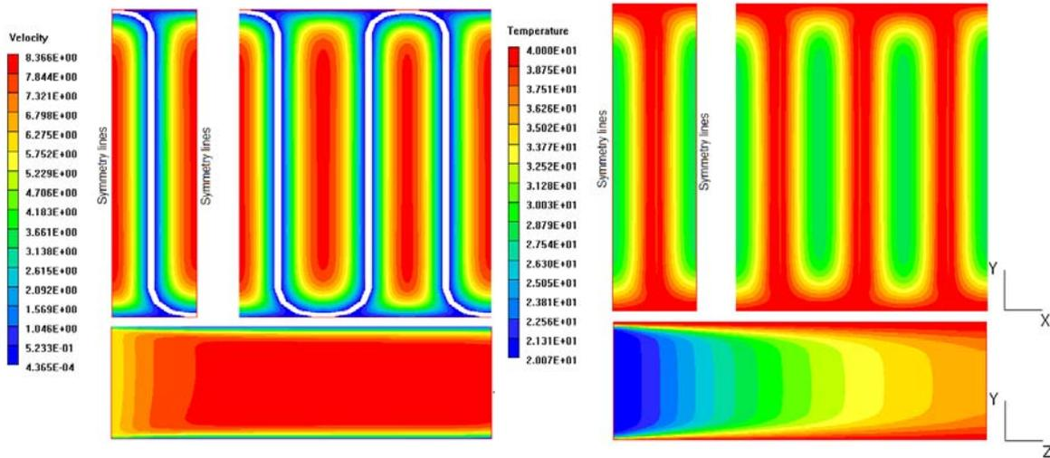
Figure 5. Profile of velocity and temperature to the laminar flow in model 15.08 ( $X = 0$  and  $Z = 0,05m$ ).
