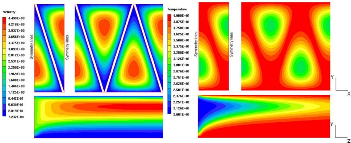
Figure 4. Profile of velocity and temperature to the laminar flow in model 11.94T ( $X = 0$  and  $Z = 0,05m$ ).
