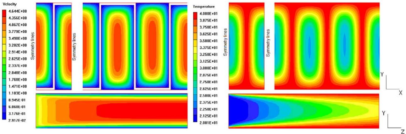
Figure 3. Profile of velocity and temperature to the laminar flow in model 6.2 ( $X = 0$  and  $Z = 0,1m$ ).
