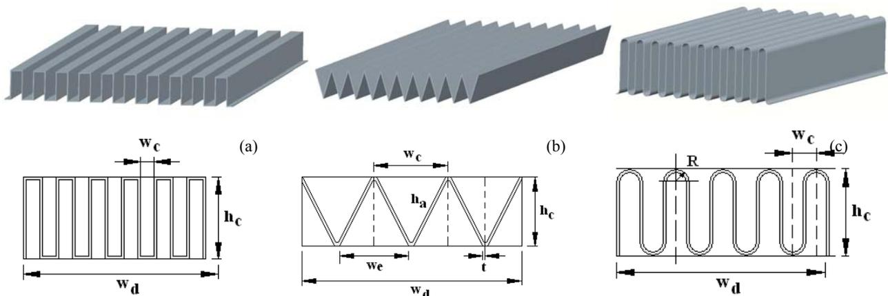
Figure 1. Ducts tested: (a) 6.2, (b) 11.94T e (c) 15.08.
