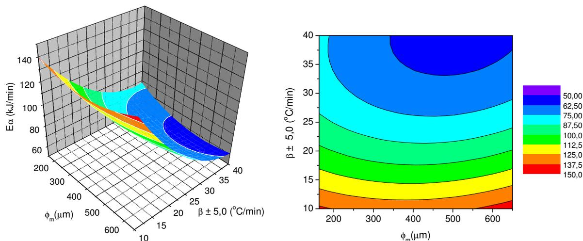
Figure 4. Response surface and contour curves for the char combustion to coal EC4500.
