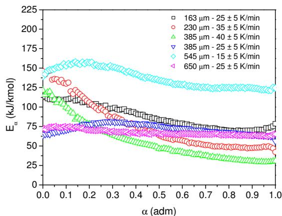
Figure 3. Activation energy ( $E_a$ ) against conversion ( $\alpha$ ) along the second region of coal combustion (char combustion) to EC4500.  $E_a$  values considering three tests on  $\beta \pm 5$  °C/min were obtained.
