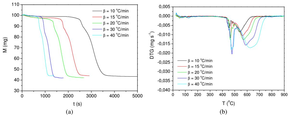
Figure 1. Effect of heating rate ( $\beta$ ) in the decomposition of coal EC4500 with an average particle size of  $385 \mu\text{m}$ : (a) TG curves and (b) DTG curves.
