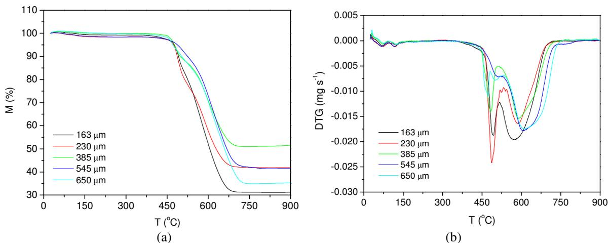
Figure 2. Effect of average particle size ( $\phi_m$ ) curves of coal combustion EC4500 with  $\beta = 30^\circ\text{C}/\text{min}$ : Profiles (a) TG and (b) DTG as a function of temperature.
