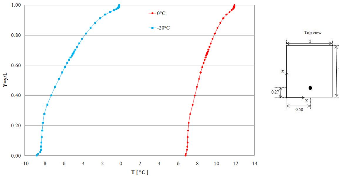
Figure 5. Temperature distribution in the  $y$  direction in the plane  $X = 0.58$  and  $Z = 0.27$  for  $T_e = 0^\circ\text{C}$  and  $T_e = -20^\circ\text{C}$ .
