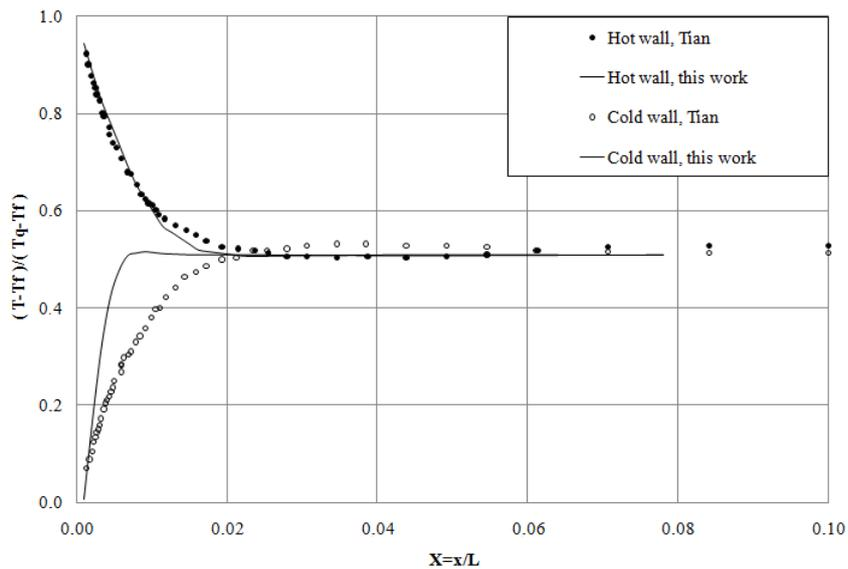
Figure 4. Comparison of the temperature distribution near the walls at  $Y=0.5$ .
