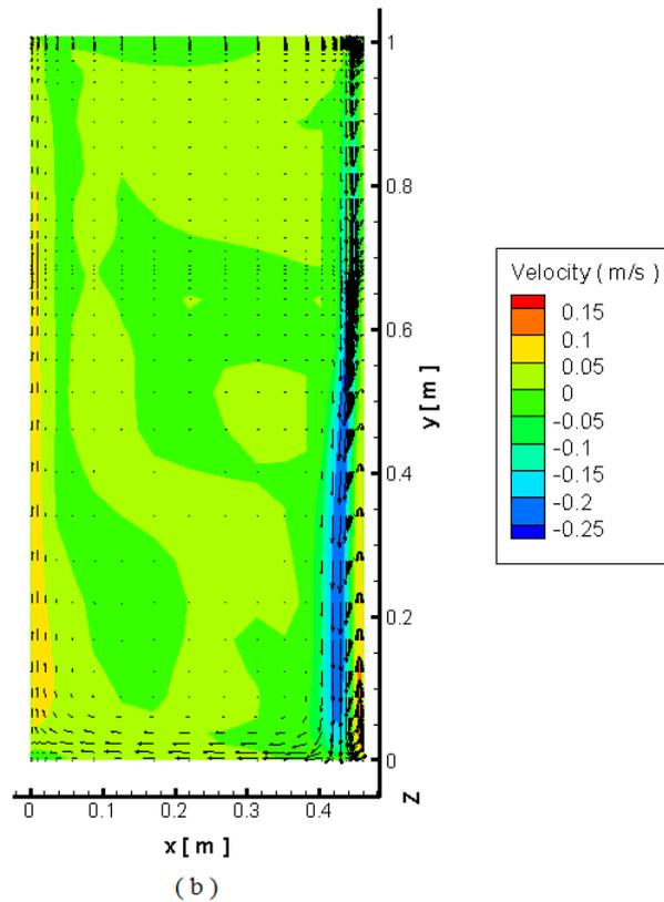
Figure 6. (a) Temperature and (b) velocity fields for  $T_e = -15^\circ\text{C}$  for  $z = 0.259$  m (continuation).
