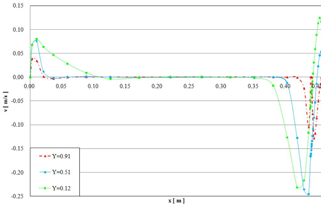
Figure 8: Velocity distribution for  $T_e = -15^\circ\text{C}$  at  $z = 0.582\text{ m}$ .
