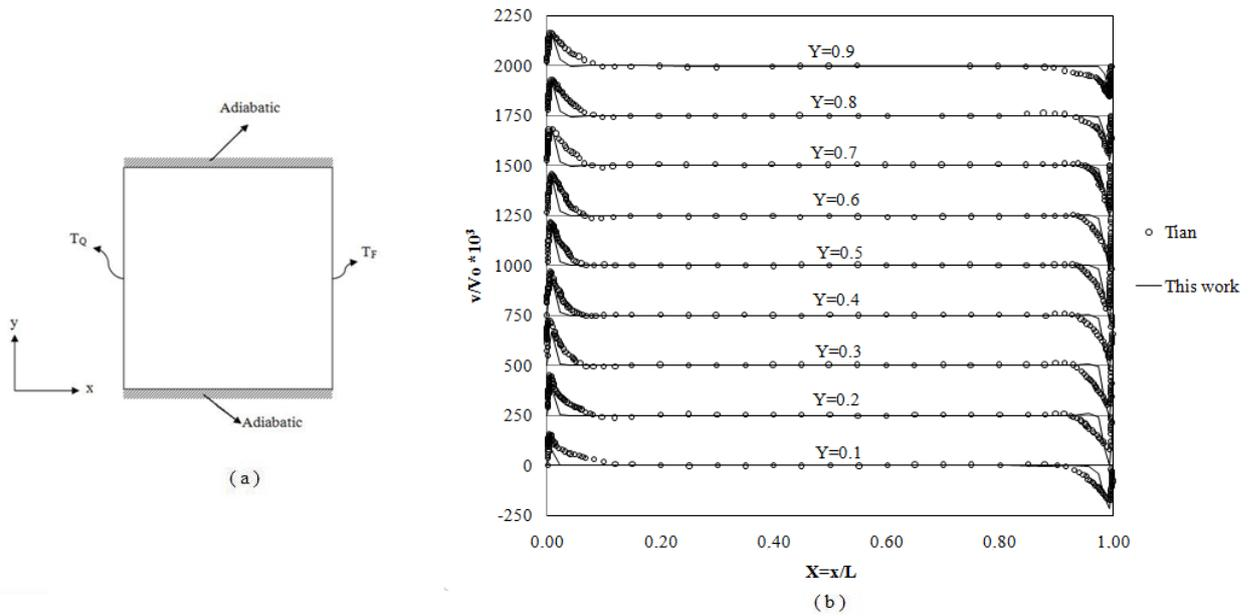
Figure 3. (a) Schematic of the air filled square cavity and (b) Vertical velocity distribution at different heights.
