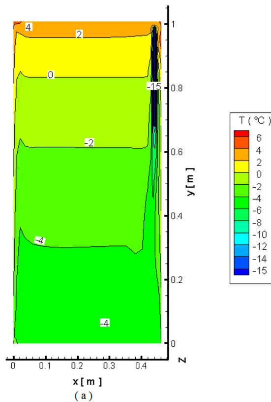
Figure 6. (a) Temperature and (b) velocity fields for  $T_e = -15^\circ\text{C}$  for  $z = 0.259$  m.
