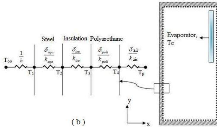
Figure 1. (a) Geometry of the cabinet and (b) Thermal resistances between the external environment and the interior of the cabinet (continuation).
