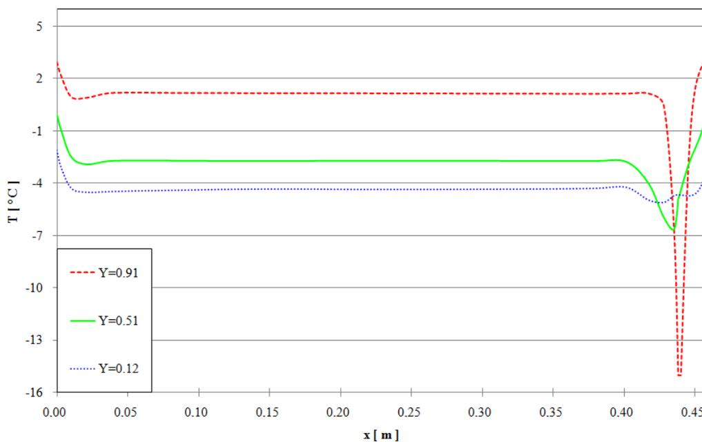
Figure 7: Temperature distribution for  $T_e = -15^\circ\text{C}$  in the direction at  $z = 0.582$  m.
