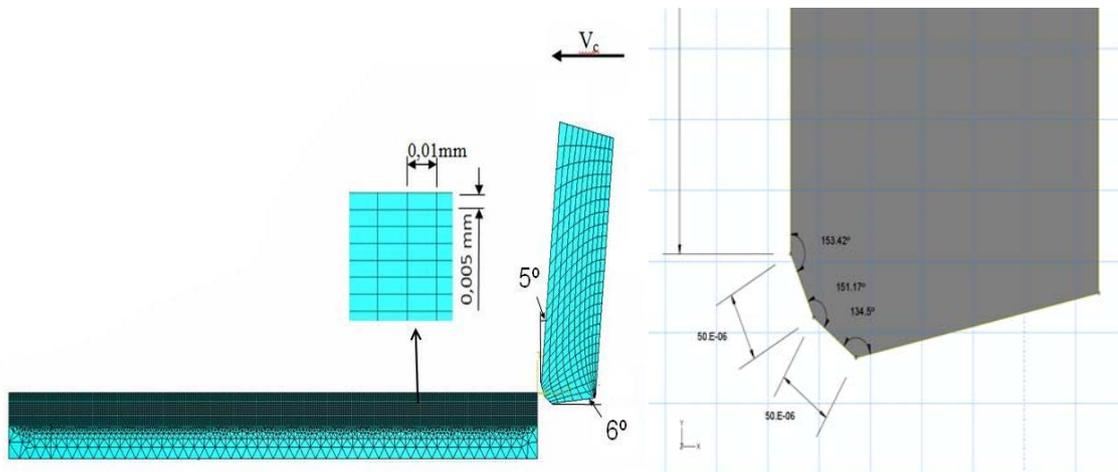
Figure 1: Workpiece and Insert dimensions
