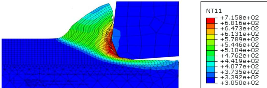
Figure 3. ABAQUS Temperature Simulation
