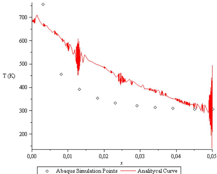
Figure 5. Simulation versus Analytical temperature at 30 s for several point on the workpiece
