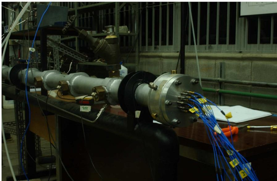
Figure 1. Shock tube T1 with 21 PCB sensors at the end of the low-pressure reservoir.
