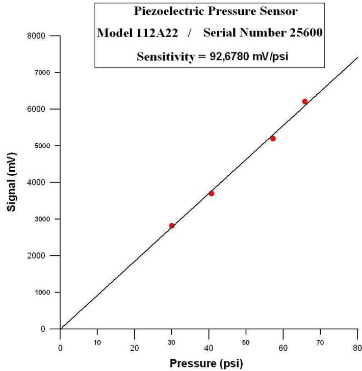
Figure 5. Calibration curve for sensor number 1
