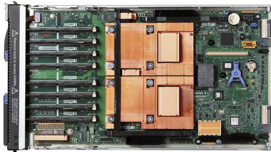
Figure 4. Typical blade with two microprocessors and a heat generation capacity higher than 300W.
