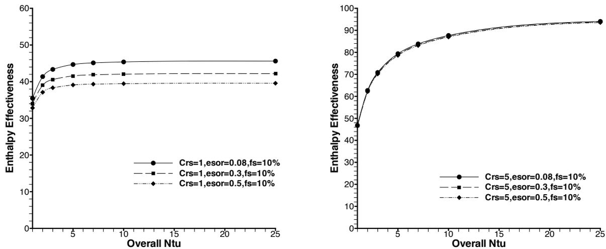
Figure 3. Variation of  $\varepsilon_i(\%)$  with overall  $N_{tu}$ s for and  $f_s = 10\%$  for different heats of sorption.
