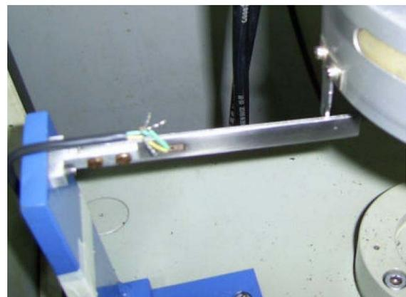
Figure 7. Standard calibration test of a strain gage.
