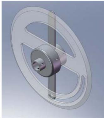
Figure 11. SolidWork modeling of the angle-of attack protractor.
