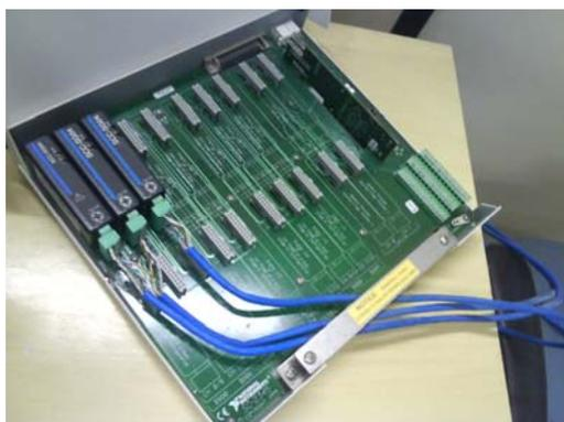
Figure 20. Connector block SC-2345.
