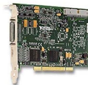
Figure 21. Data acquisition board PCI-6221.
