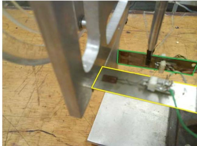
Figure 5. Zoom into the lift and pitching-moment strain-gage mounting.
