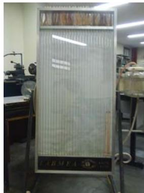
Figure 19. Multitube variable inclination manometer.
