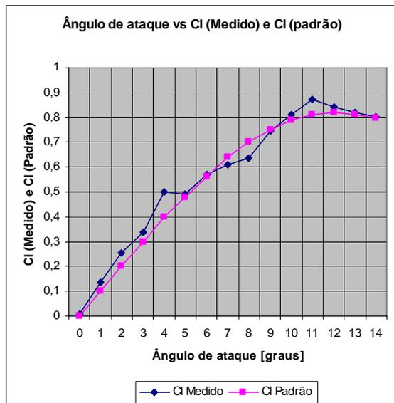
Figure 25. Comparison with the NACA data (Blevins, 1984): lift coefficient
