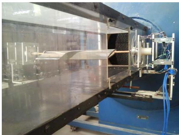
Figure 2. Front view of the general balance assembly in the wind tunnel.
