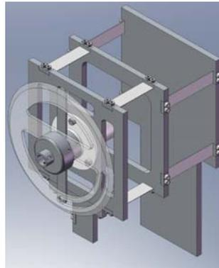
Figure 12. SolidWork modeling of the angle-of attack measuring system.
