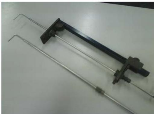
Figure 18. Pitot-static tube.
