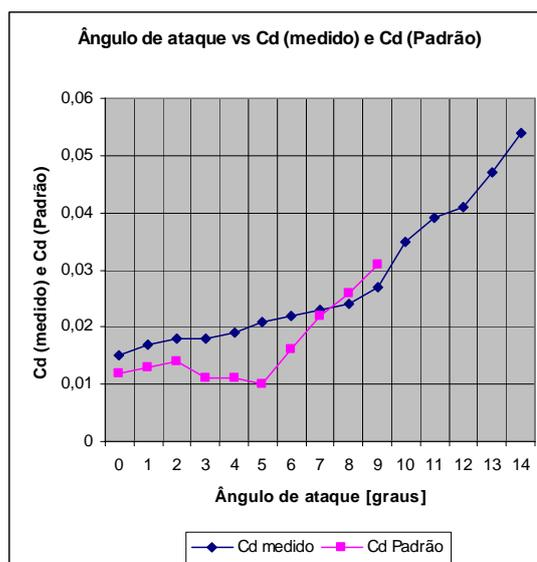
Figure 26. Comparison with the NACA data (Blevins, 1984): drag coefficient
