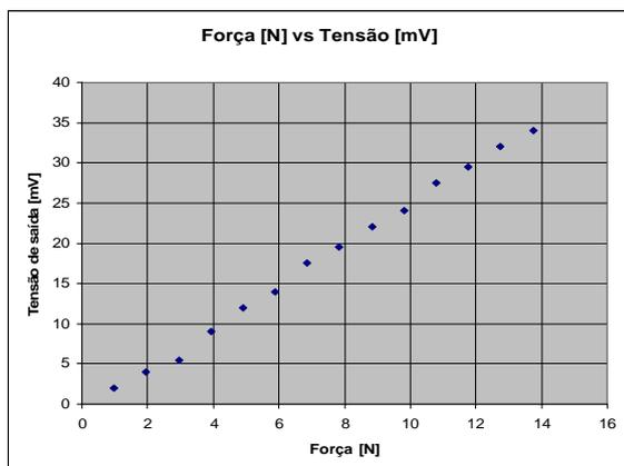
Figure 6. Calibration curve of a strain gage.
