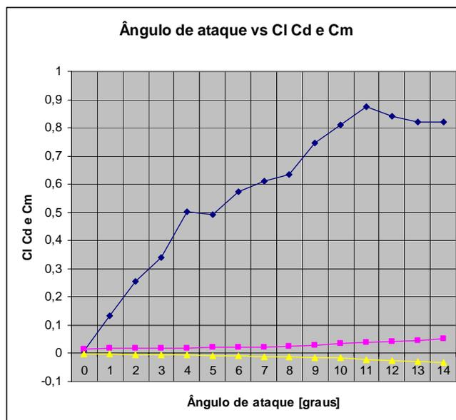
Figure 24. Measured data for the lift, drag and pitching moment coefficients as a function of the angle of attack.
