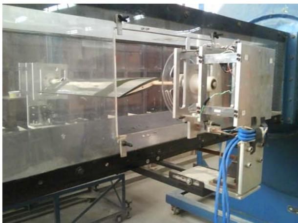
Figure 1. Skewed view of the general balance assembly in the wind tunnel.
