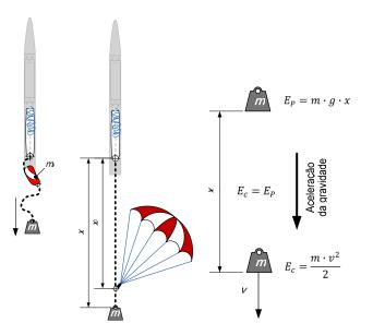
Figure 8. Determination of the energy to extend the recovery system
