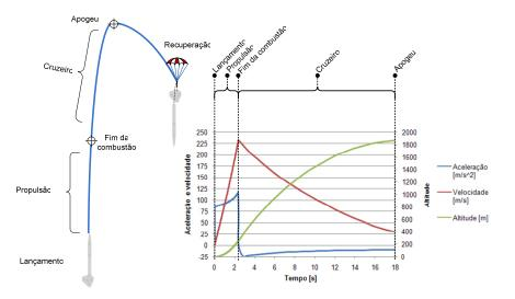
Figure 9. Free flight rocket main events and the relation with aceleration, speed and altitude.
