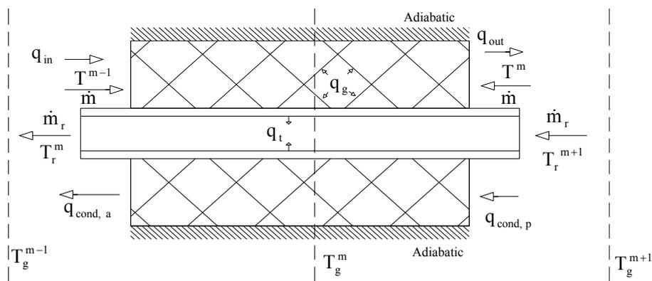
Figure 6. Heat and mass transfer interactions in cell "m"
