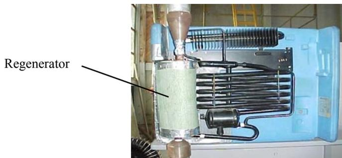
Figure 3. Location of the regenerator in the prototype.
