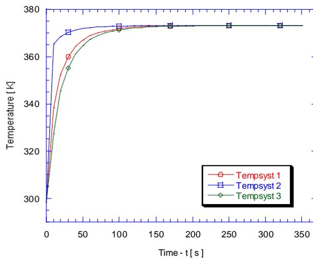
Figure 13. Temperature transient evolution in the first cell  $\phi = 0.8$ ;  $L = 1$  m;  $\dot{m} = 0.1$  kg/s.
