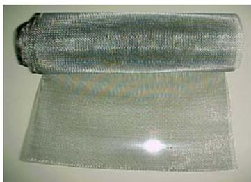
Figure 2. The metallic aluminum grid utilized to assemble the metallic matrix.
