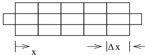
Figure 5. Heat exchanger divided in volume elements.
