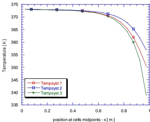
Figure 10. Steady state temperature values for  $\phi = 0.5$ ;  $L = 1$  m;  $\dot{m} = 0.1$  kg/s.
