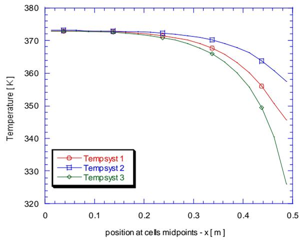
Figure 12. Steady state temperature values for  $\phi = 0.8$ ;  $L = 0.5$  m;  $\dot{m} = 0.1$  kg/s.
