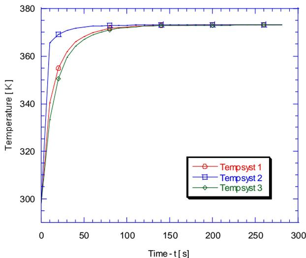
Figure 11. Temperature transient evolution in the first cell for  $\phi = 0.8$ ;  $L = 0.5$  m;  $\dot{m} = 0.1$  kg/s.
