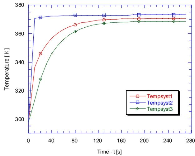
Figure 7. Temperature transient evolution in the first cell for  $\phi = 0.95$ ;  $L = 1$  m;  $\dot{m} = 0.1$  kg/s.
