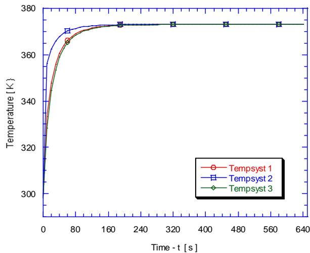
Figure 9. Temperature transient evolution in the first cell for  $\phi = 0.5$ ;  $L = 1$  m;  $\dot{m} = 0.1$  kg/s.
