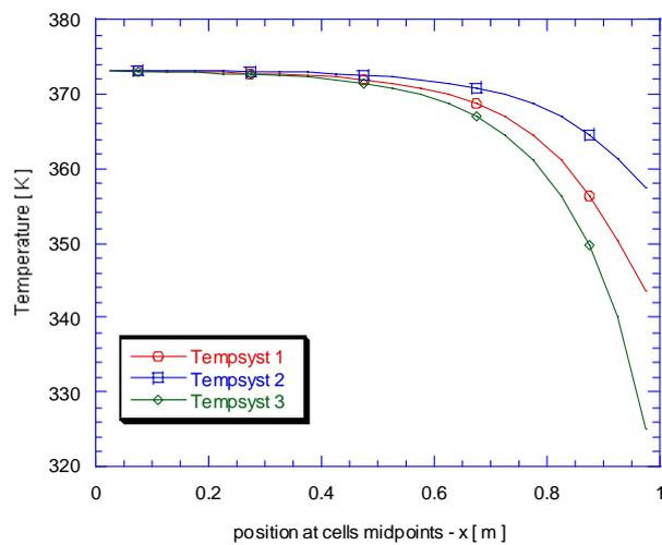
Figure 14. Steady state temperature values for  $\phi = 0.8$ ;  $L = 1$  m;  $\dot{m} = 0.1$  kg/s.
