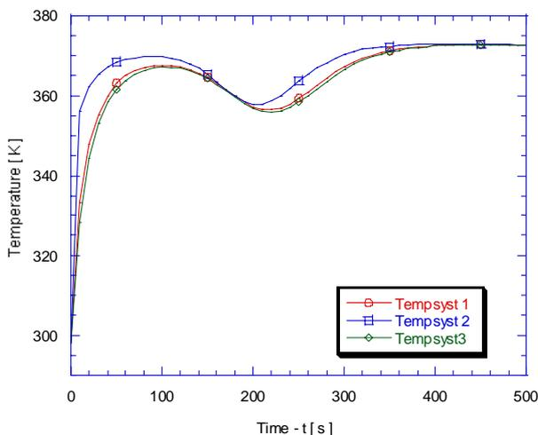
Figure 15. Temperature transient evolution in the first cell for  $\phi = 0.5$ ;  $L = 1$  m;  $\dot{m} = f(t)$ .
