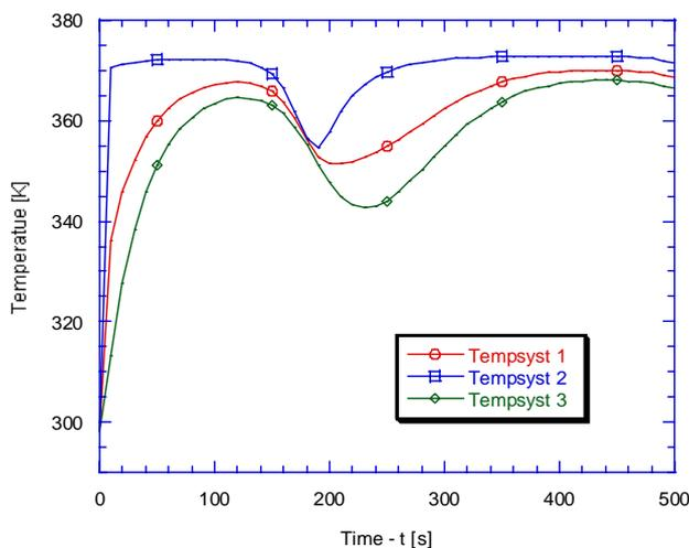
Figure 16. Steady state temperature values for  $\phi = 0.95$ ;  $L = 1$  m;  $\dot{m} = f(t)$ .
