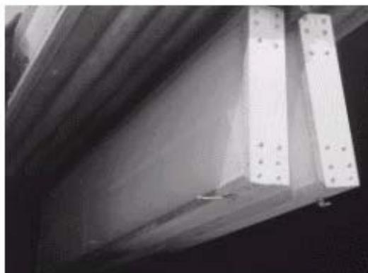
Fig. 9. TIM covers positioned during the refrigeration stage.
