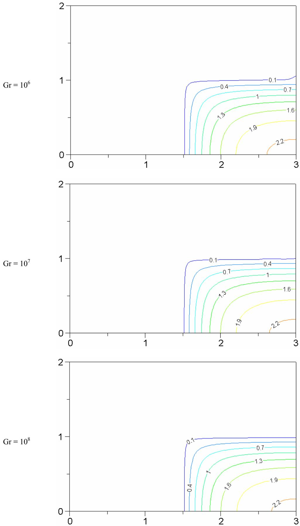
Figure 4. Numerically simulated isoconcentration lines for  $Gr = 10^6$ ,  $10^7$  and  $10^8$ .
