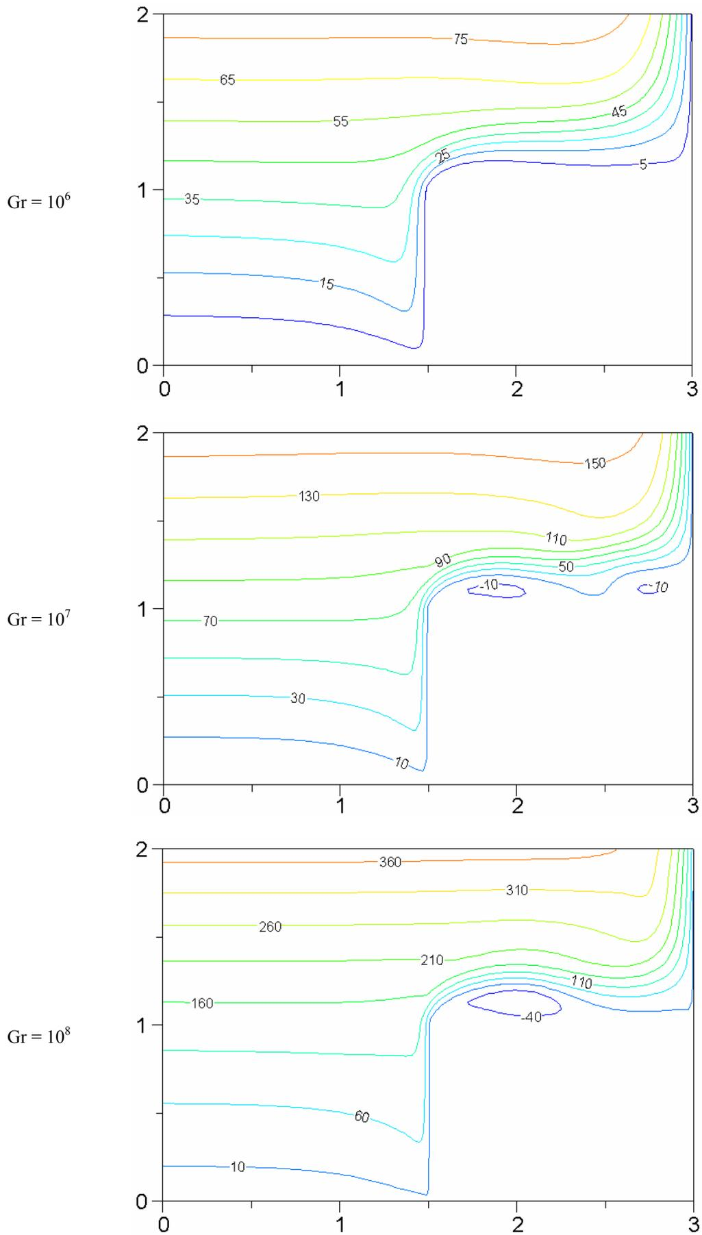
Figure 2. Numerically simulated streamlines for  $Gr = 10^6$ ,  $10^7$  and  $10^8$ .
