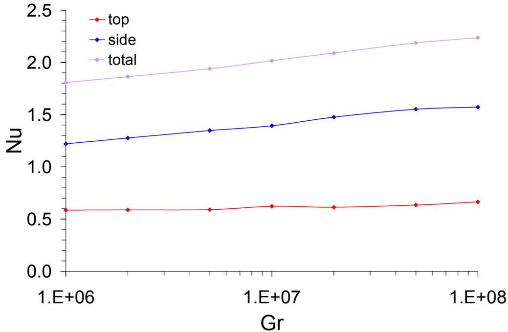
Figure 5. Average Nusselt number (at the stack top, at the stack left side and total) as a function of Grashof number.
