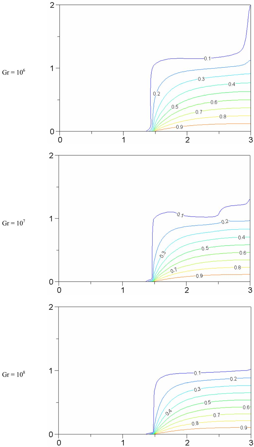
Figure 3. Numerically simulated isotherms for  $Gr = 10^6, 10^7$  and  $10^8$ .
