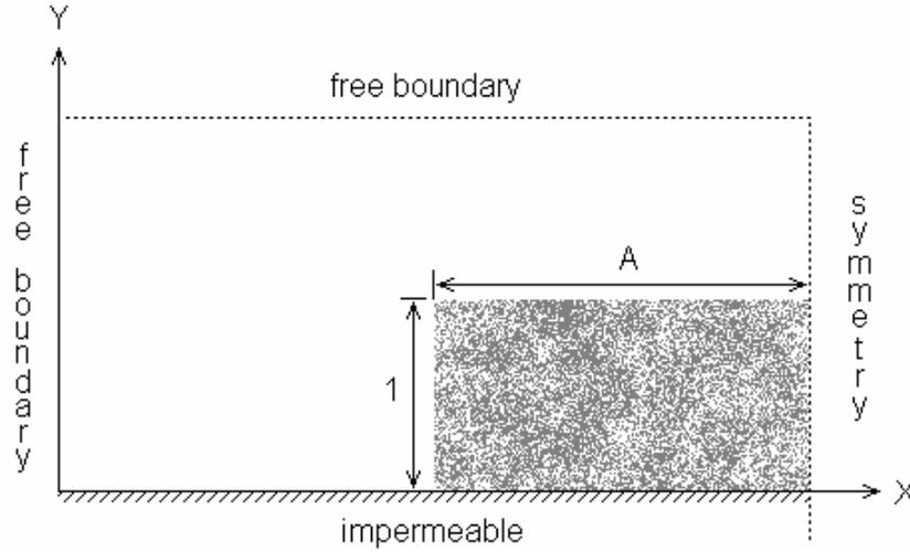
Figure 1. Schematic diagram of the rectangular shaped phosphogypsum stack investigated.
