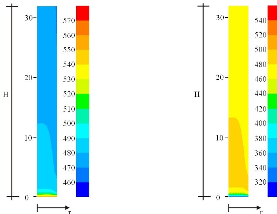
Figure 7. Bi-dimensional temperature profiles: (a) gaseous phase (b) solid phase
