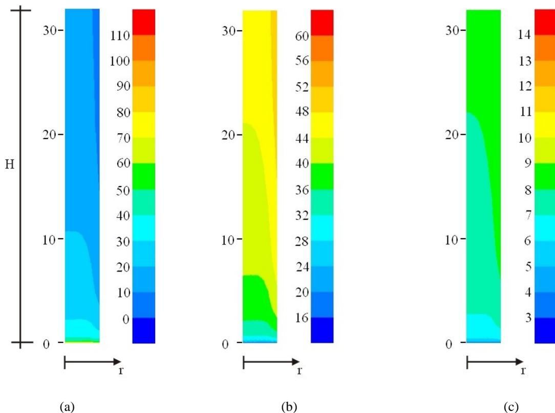
Figure 5. Lumps concentrations along the riser for: (a) gasoil, (b) gasoline and (c) LPG
