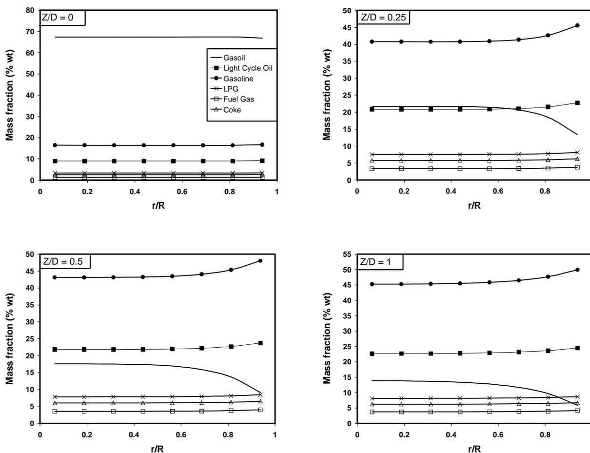
Figure 6. Radial mass fraction profiles for various cross sections along the riser
