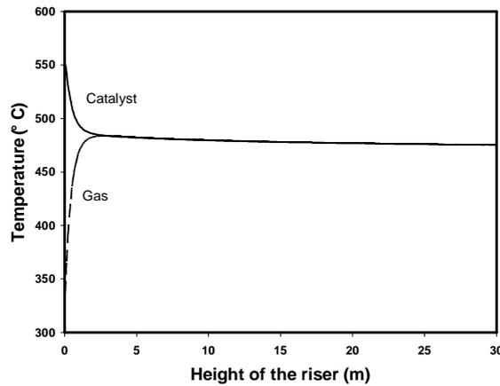
Figure 4. Average temperature profiles along the riser
