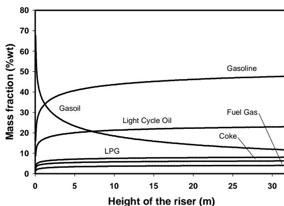
Figure 3. Mass fraction profiles along the riser
