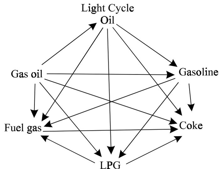
Figure 2. Lumped kinetic scheme
