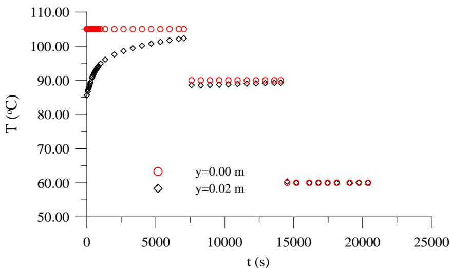
Figure 5. Air temperature within the bed during fresh cocoon drying process.
