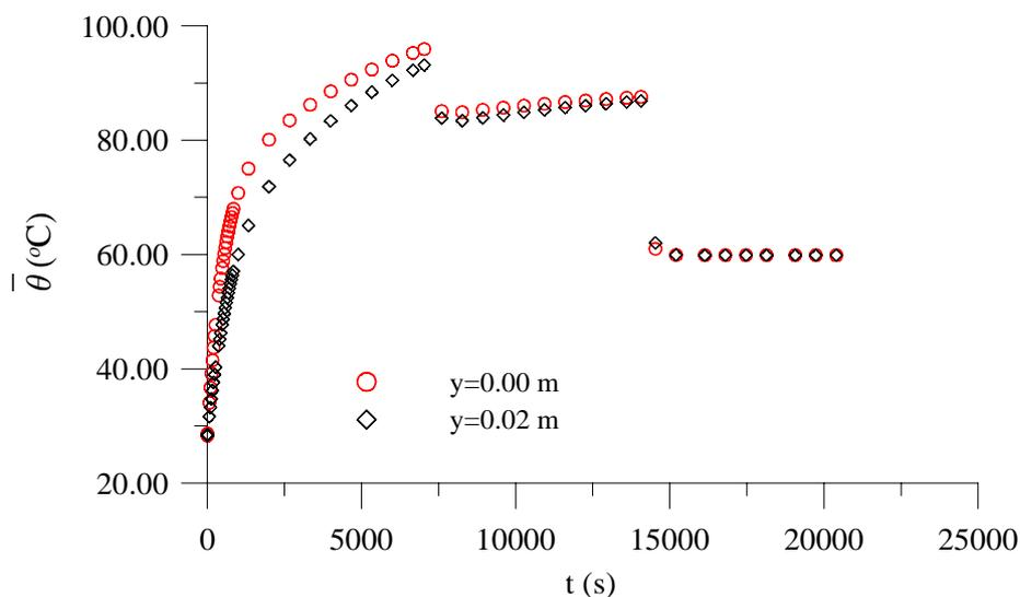
Figure 6. Cocoon temperature within the bed during drying process.
