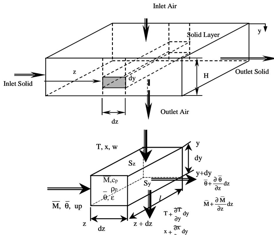
Figure 2. Schematic representation of the multi-zone cross flow belt conveyor dryer.
