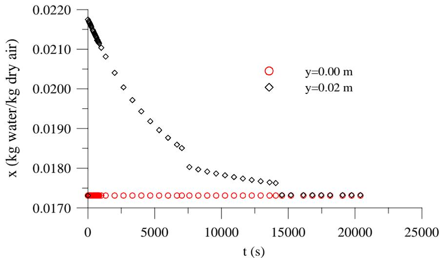
Figure 7. Air absolute humidity within the bed along drying process.
