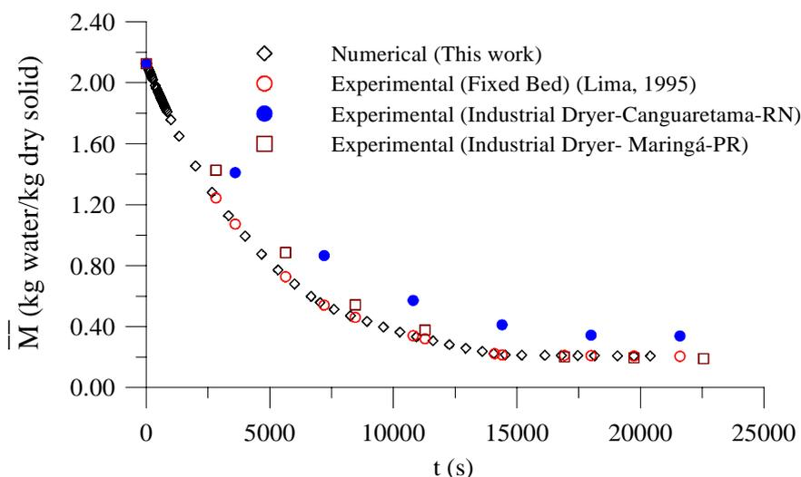
Figure 4. Comparison between the predicted and experimental values of the moisture content during drying process of fresh cocoon to  $H = 0.02\text{m}$
