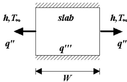
Figure 2 - Heat Generating Vertical Slab
