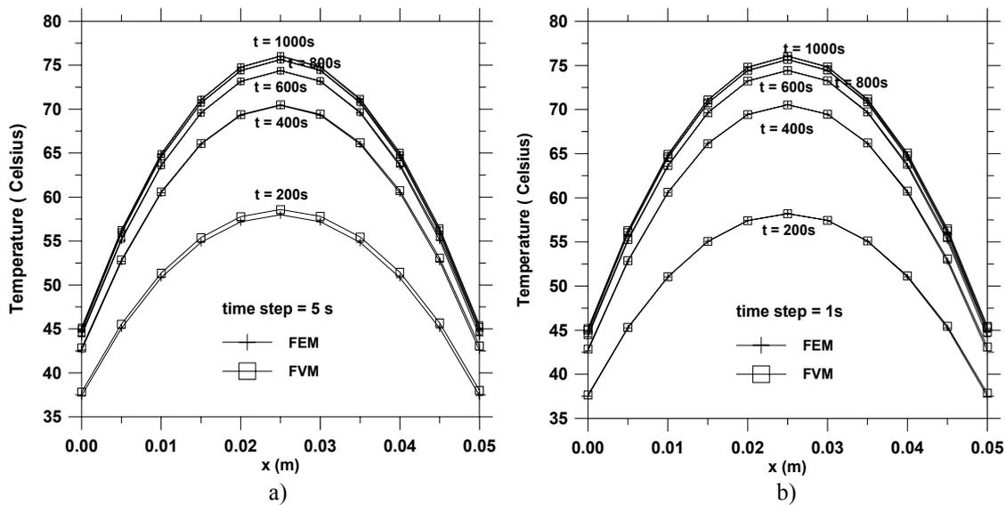
Figure 5 - Temperature profile as a function of x for several time instants: (a) for time step equal to 5 s and (b) for time step equal to 1 s.
