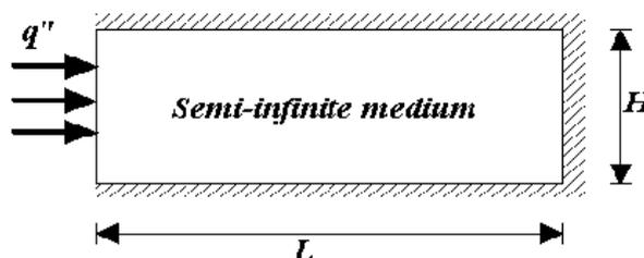
Figure 1 - Semi-Infinite Medium
