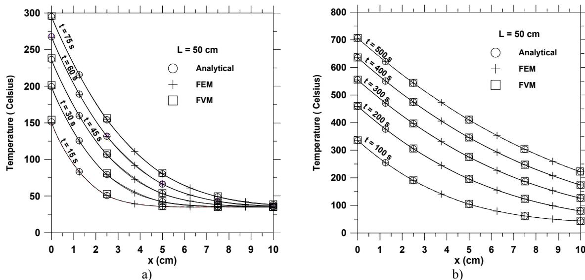
Figure 4 - Temperature profile as a function of x for different time instants: (a) from 15 to 75 s and (b) from 100 to 500 s.
