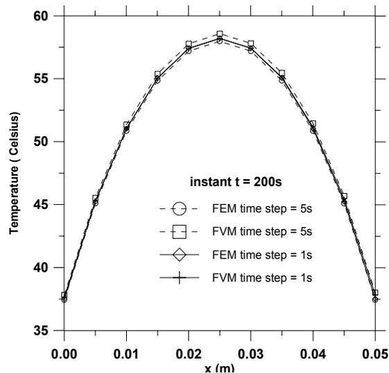
Figure 6 - The temperature profile at 200 s obtained by the two methods for time steps of 5 and 1 s.
