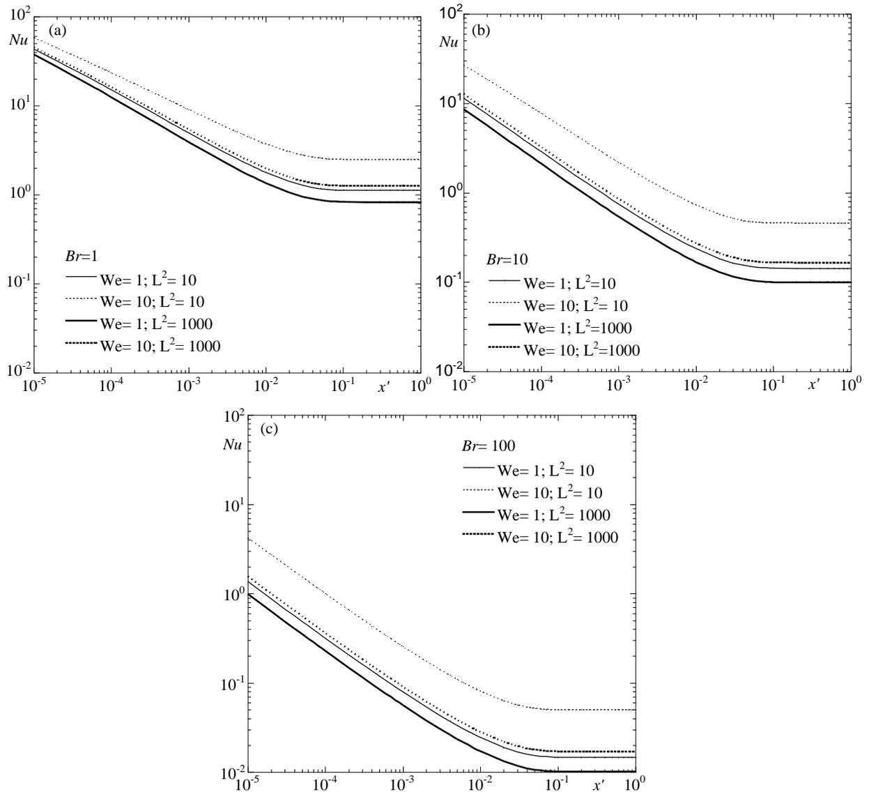
**Figure 2-** Effect of viscoelasticity, measured by  $We$  and  $L^2$ , on the Nusselt number variation for various Brinkman numbers, and for wall heating ( $\dot{q}_w > 0$ ): (a)  $Br = 1$ ; (b)  $Br = 10$ ; (c)  $Br = 100$ .
