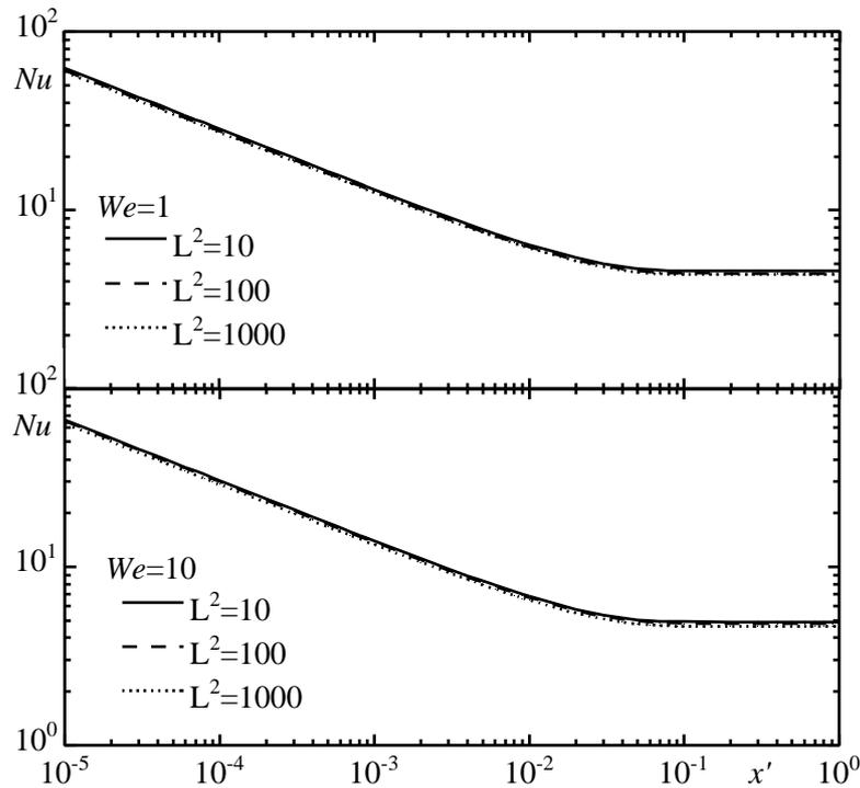
Figure 1- Effect of viscoelasticity, measured by  $We$  and  $L^2$ , on the Nusselt number variation in the absence of viscous dissipation ( $Br=0$ ).
