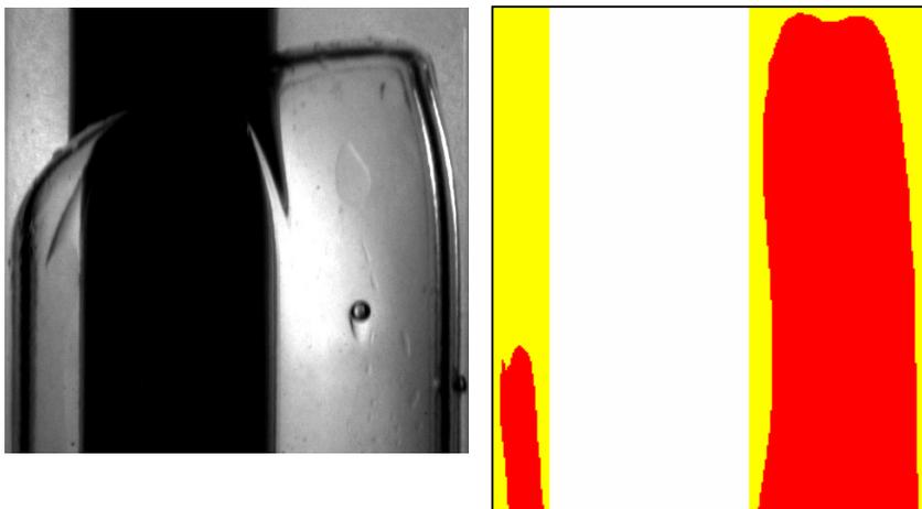
Figure 11. Carbopol 0.15%wt displacing Oil
