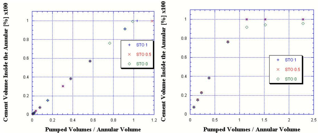
Figures 7 and 8 – Process efficiency. Cement displacing spacer in 1 and 10 BPM for three eccentricities.
