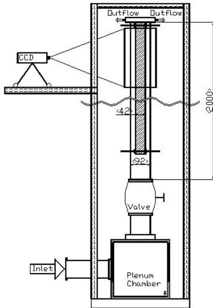
Figure 1 – Experimental Apparatus
