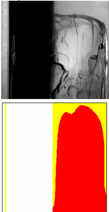
Figure 9. Carbopol 0.15%wt displacing Oil
