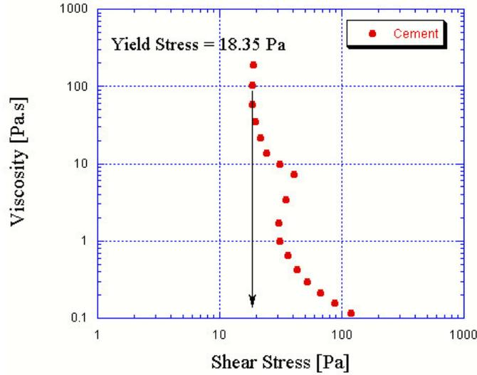
Figure 4. Viscosity x Shear Stress – Cement Yield Stress
