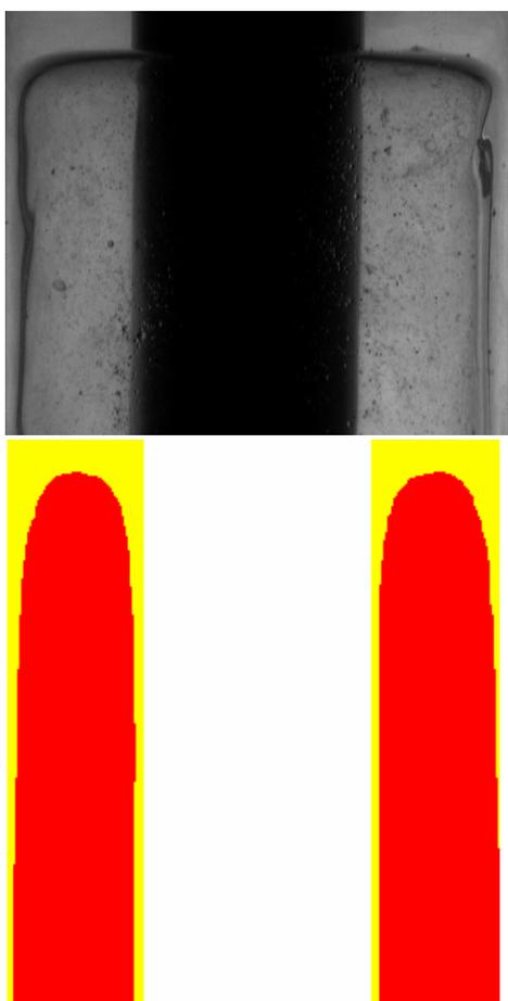
Figure 12. Carbopol 0.15%wt displacing Oil
