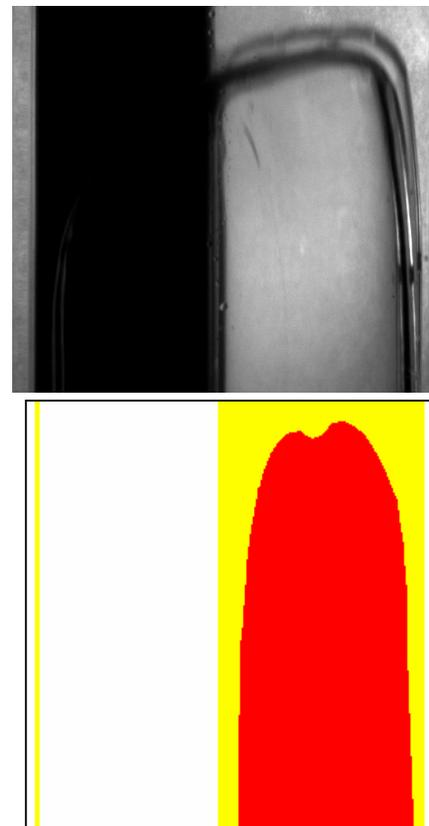
Figure 10. Carbopol 0.15%wt displacing Oil
