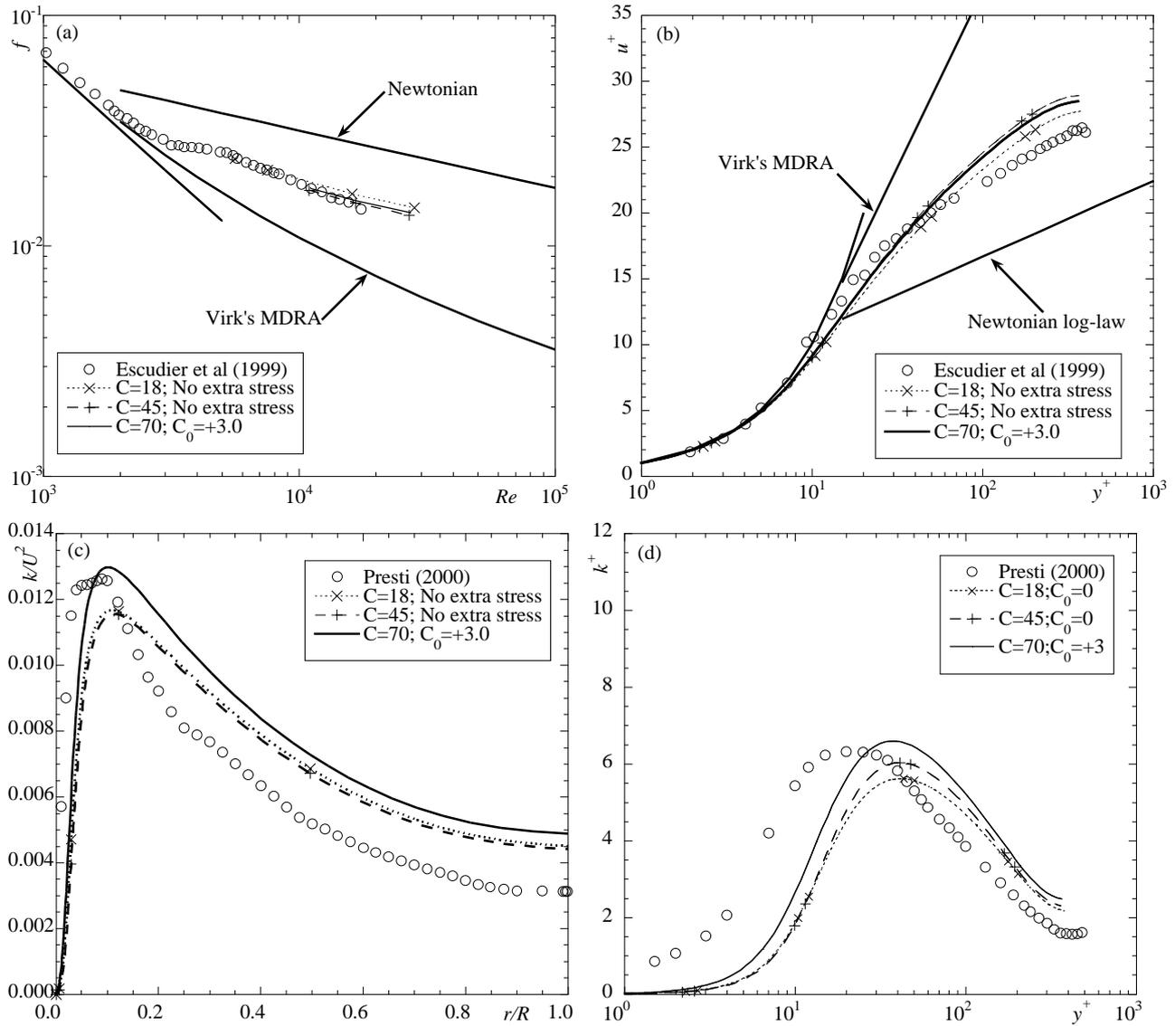
Figure 3- Predictions of flow of 0.25% CMC at  $Re= 16,600$  with new stress ( $C= 70$  and  $C_0= +3.0$ ) and comparisons with model of Cruz and Pinho (2003) (old:  $C= 18$  and  $C_0= +0.0$ ), (corrected:  $C= 45$  and  $C_0= +0.0$ ) and experimental data: (a) friction factor; (b)  $u^+$  versus  $y^+$ ; (c)  $k/U^2$  versus  $r/R$ ; (d)  $k^+$  versus  $y^+$ .
