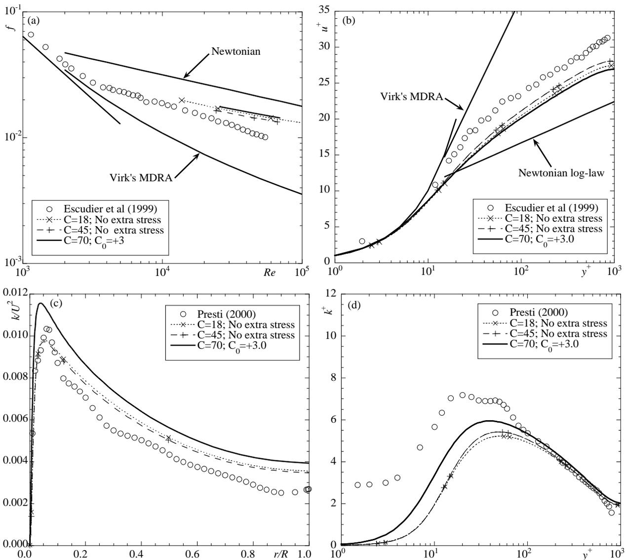
Figure 4- Predictions of flow of 0.09%/0.09% CMC/XG at  $Re=45,300$  with the model with new stress ( $C=70$  and  $C_0=+3.0$ ) and comparisons with model of Cruz and Pinho (2003) (old:  $C=18$  and  $C_0=+0.0$ ), (corrected:  $C=45$  and  $C_0=+0.0$ ) and experimental data: (a) friction factor; (b)  $u^+$  versus  $y^+$ ; (c)  $k/U^2$  versus  $r/R$ ; (d)  $k^+$  versus  $y^+$ .
