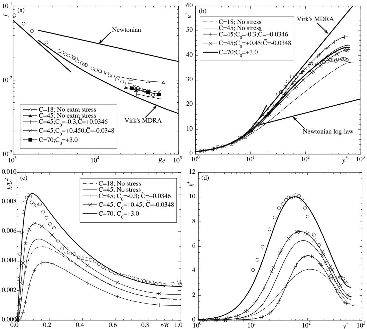
Figure 1- Effect of  $C$  and of new stress on flow for 0.125% PAA solution. Open circles: experimental data of Escudier et al (1999) (a,b) and Presti (2000) (c,d): (a) Friction factor; (b) Mean velocity at  $Re=42,900$ ; (c)  $k/U^2$ ; (d)  $k^+$ .
