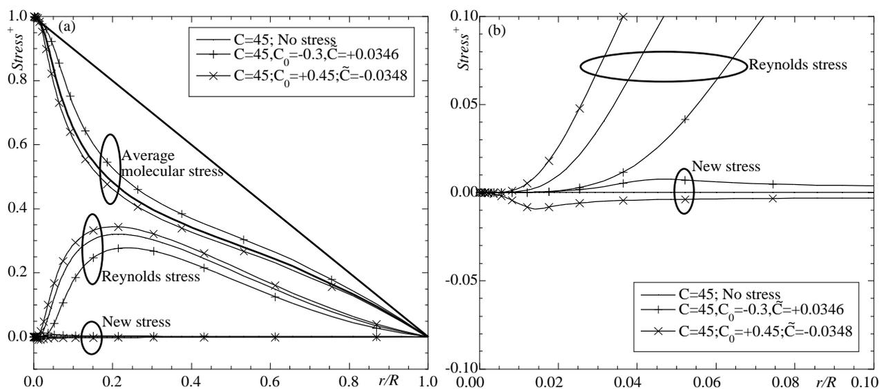
Figure 2- Effect of  $C$  and of sign of new stress on radial distribution of various shear stresses across the pipe for flow of 0.125% PAA at  $Re=42,900$ . (a) radial profile; (b) zoom in the near-wall region (for  $C_0 > 0$ ,  $-2\bar{\mu}'s_{ij}$  is plotted).
