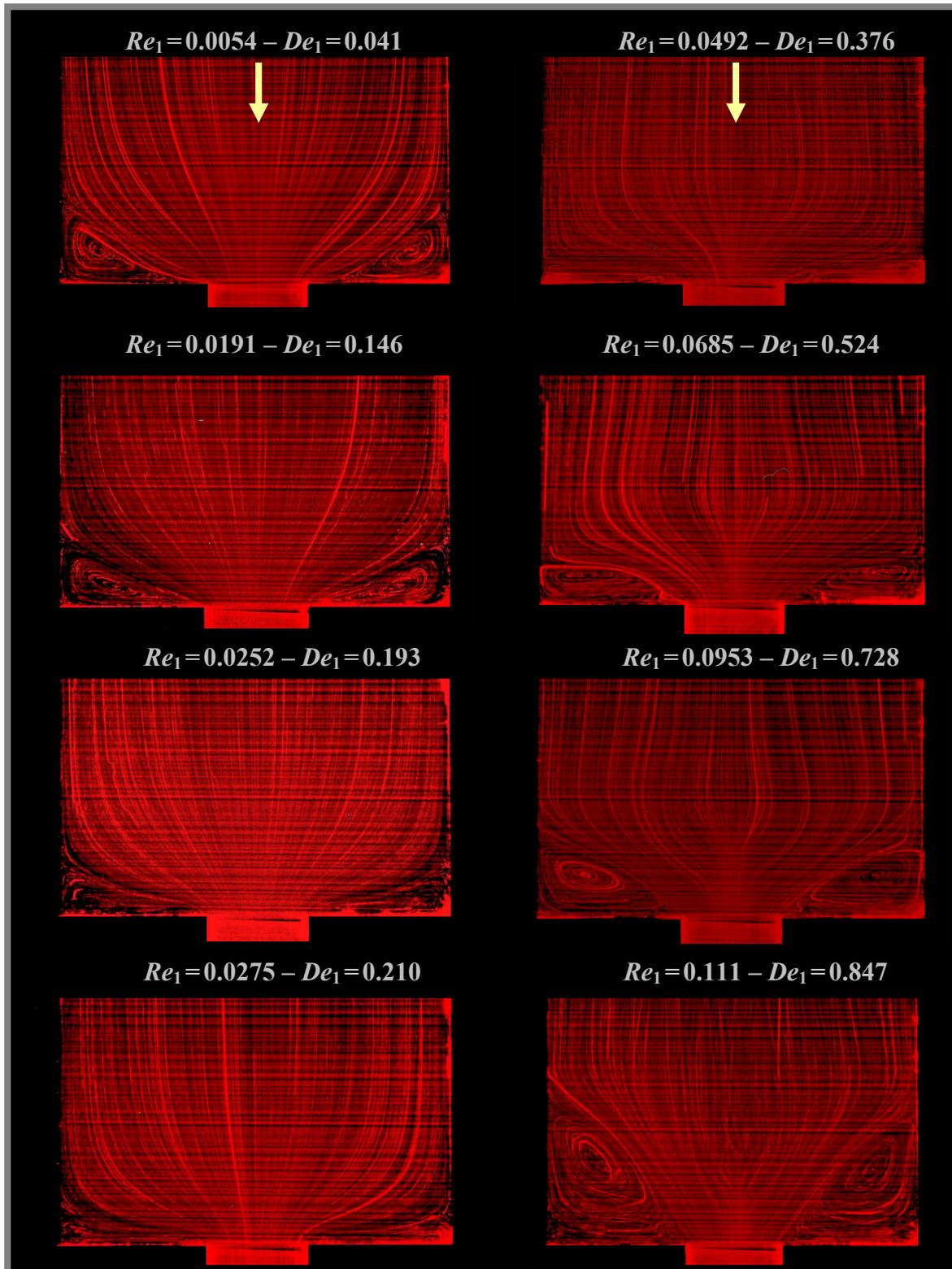
Figure 5- Influence of elasticity on the streakline flow patterns at the middle plane of a 4:1:1 sudden contraction for PAA 100.
