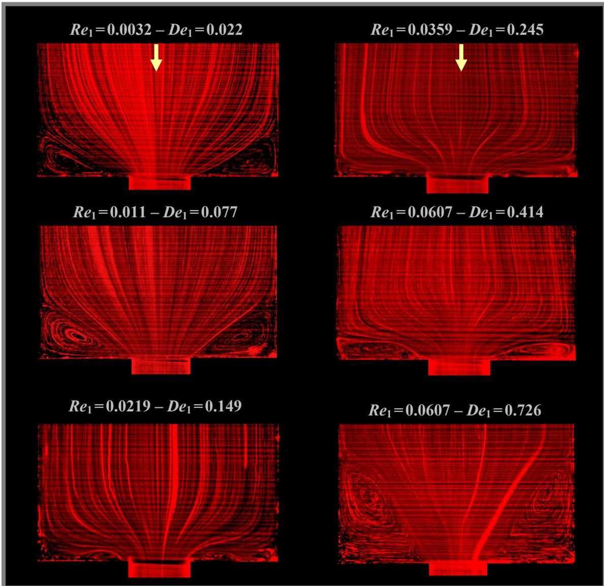
Figure 7- Influence of elasticity on the streakline flow patterns at the middle plane of a 4:1:1 contraction for PAA300.
