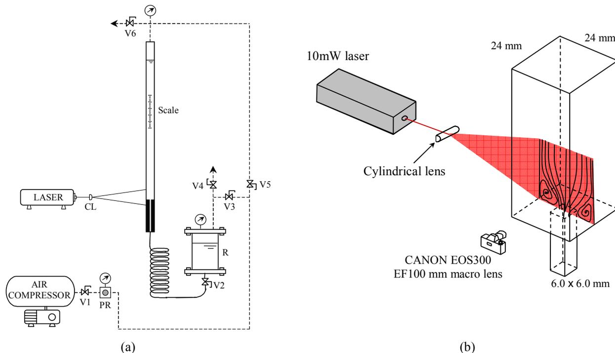
Figure 1- Experimental flow rig: (a) Schematic representation of rig (PR- pressure regulator; V1 to V6- ball valves; R- reservoir; CL- cylindrical lens); (b) Flow visualization technique and test section.
