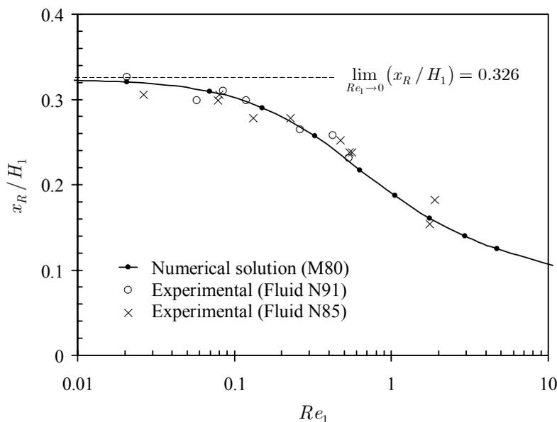
Figure 4- Influence of the Reynolds number on the vortex length at the middle plane of a square-square 4:1:1 sudden contraction for Newtonian fluids N85 and N91. Comparison between experiments and numerical predictions.
