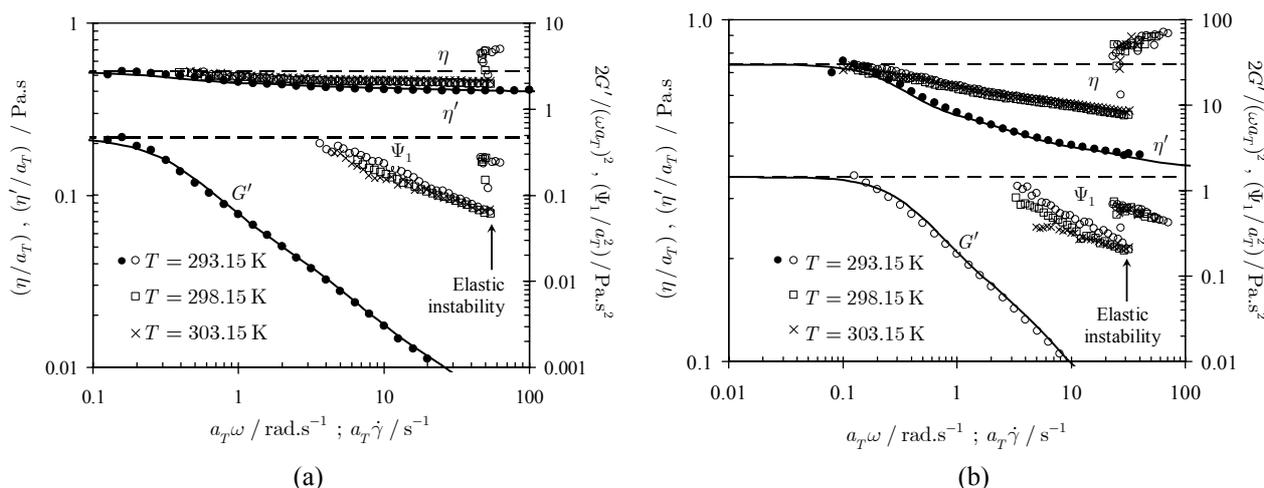
Figure 2- Material parameters in steady ( $\eta, \Psi_1$ ) and oscillating ( $G', \eta'$ ) shear flow for the Boger fluids: (a) PAA 100; (b) PAA 300. Lines represent fitting by a three-mode Oldroyd-B model.
