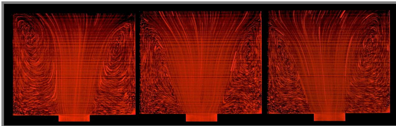
Figure 6- Streaklines for the flow of PAA 100 in the middle plane of a square-square contraction at three different moments within one different oscillating supercritical flow condition ( $De_1 = 1.22$ ).
