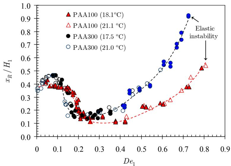
Figure 8- Variation of normalized vortex length with flow elasticity for Boger fluids PAA100 and PAA300.
