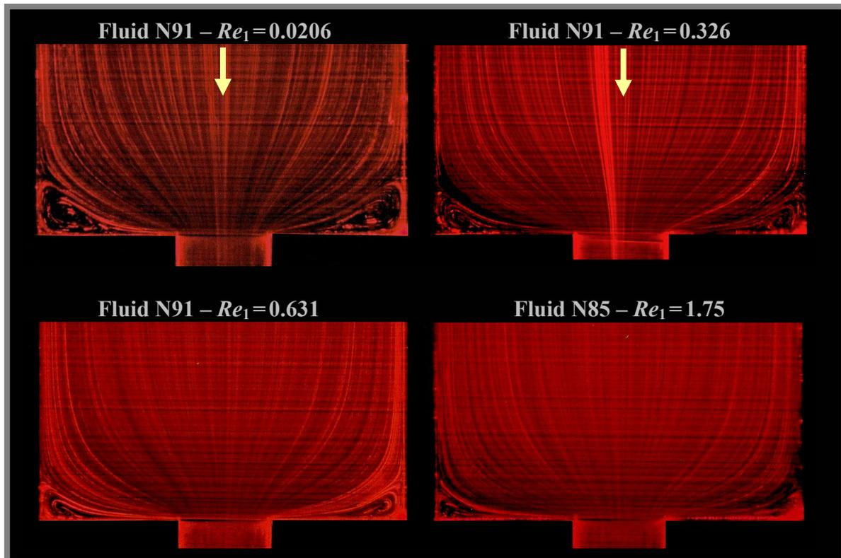
Figure 3- Streaklines for the flow of Newtonian fluids in the middle plane of a 4:1:1 sudden contraction.
