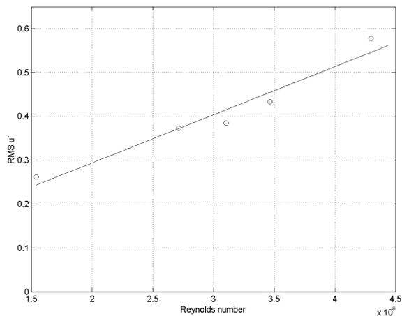
Figure 3: Turbulence intensity for non-pulsatile flows
