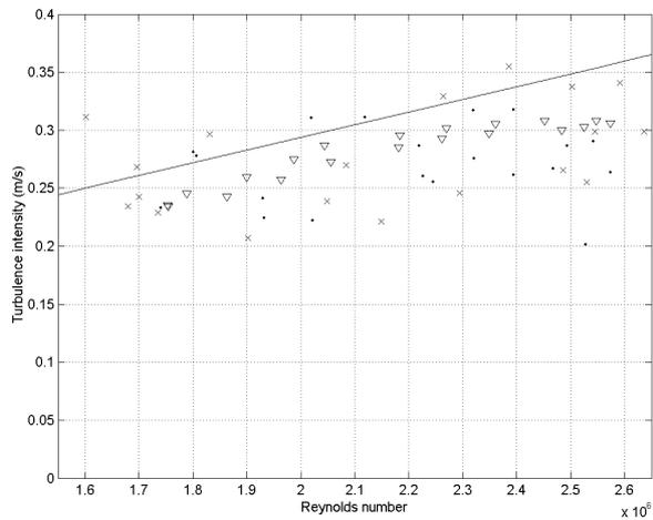
Figure 8: turbulence intensity: – non-pulsatile flow,  $\nabla$  0.33Hz,  $\times$  2Hz and  $\bullet$  3Hz pulsating flows
