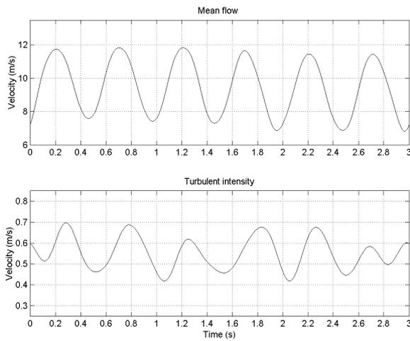
Figure 6: Mean flow and turbulence intensity -2Hz pulsation frequency
