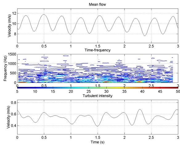
Figure 12: Time frequency analysis - 3Hz pulsating flow
