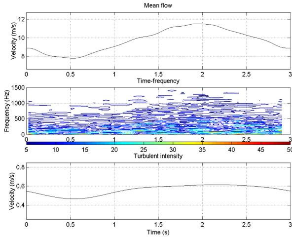
Figure 10: Time frequency analysis - 0.33Hz pulsating flow
