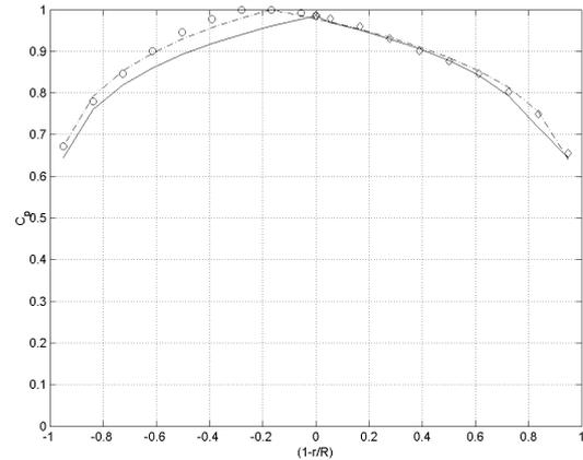
Figure 2: Velocity profile -  $\diamond$  measured values,  $\dots$  power law with  $u_c$  and  $R$  at the center,  $-\cdot-$  power law with  $u_c$  and  $R$  at the maximum velocity
