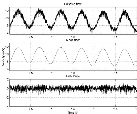
Figure 4:  $U(t)$ ,  $\bar{U}(t)$  and  $u'(t)$  for a 2Hz pulsating flow
