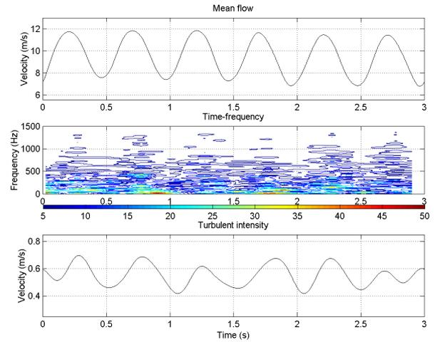
Figure 11: Time frequency analysis - 2Hz pulsating flow
