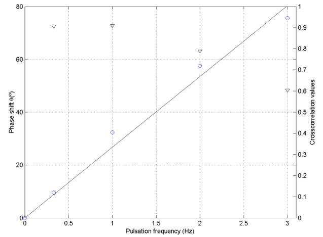
Figure 9: Phase shift between mean flow and turbulence intensity –  $\circ$  ; Cross correlation coefficient value –  $\nabla$
