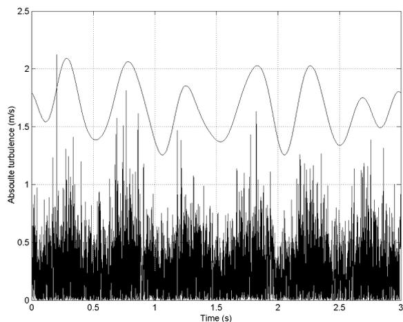
Figure 5: Turbulence intensity - 2Hz pulsation frequency
