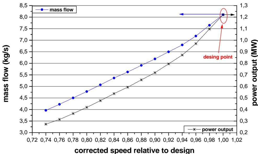
Figure 8. Air mass flow
