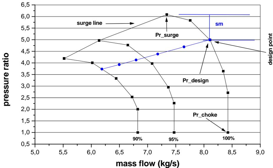
Figure 2. Compressor characteristics – surge margin definition
