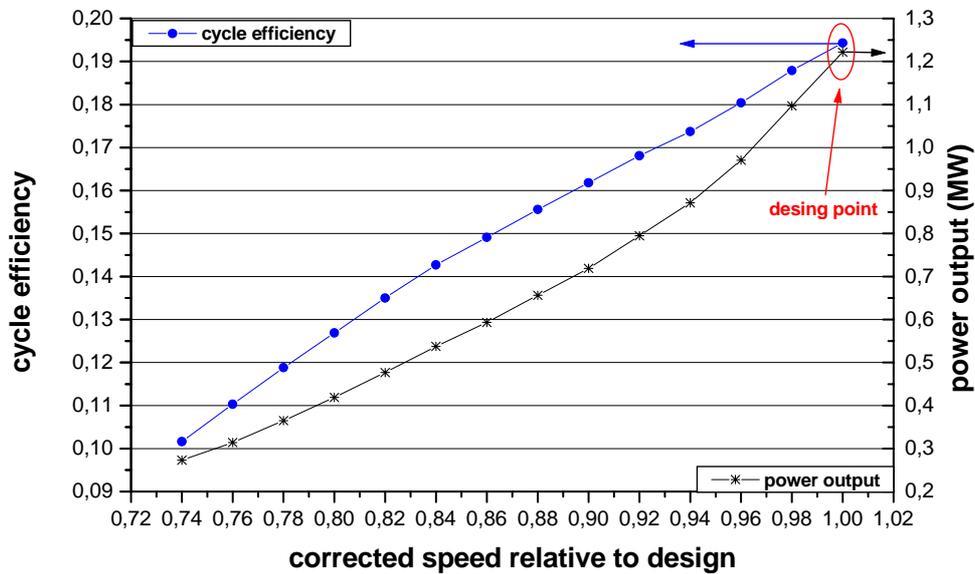
Figure 5. Cycle efficiency
