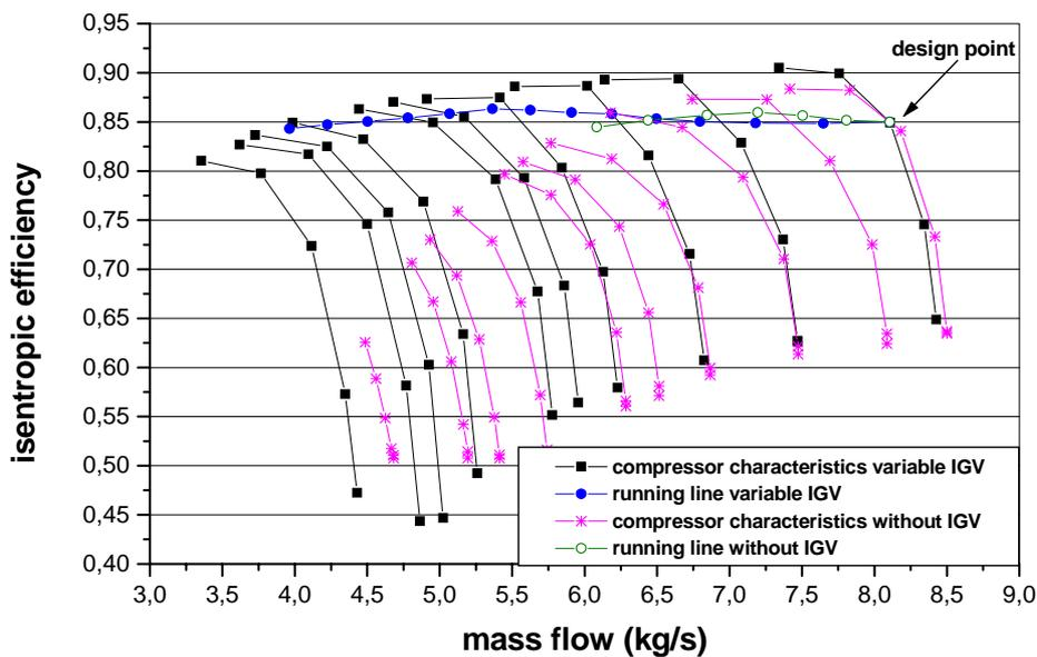
Figure 4. Compressor characteristics – isentropic efficiency
