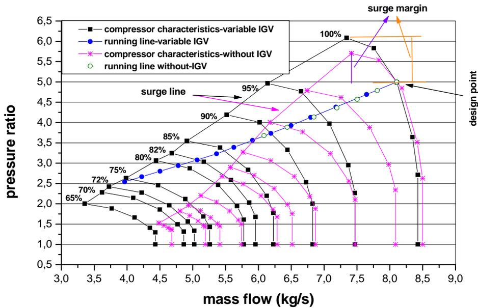
Figure 3. Compressor characteristics – pressure ratio
