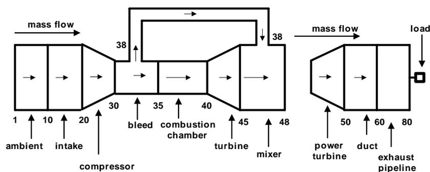
Figure 1. Sketch of a single shaft free power turbine unit
