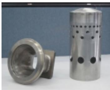
Figure 12. Combustor (liner) photo.
