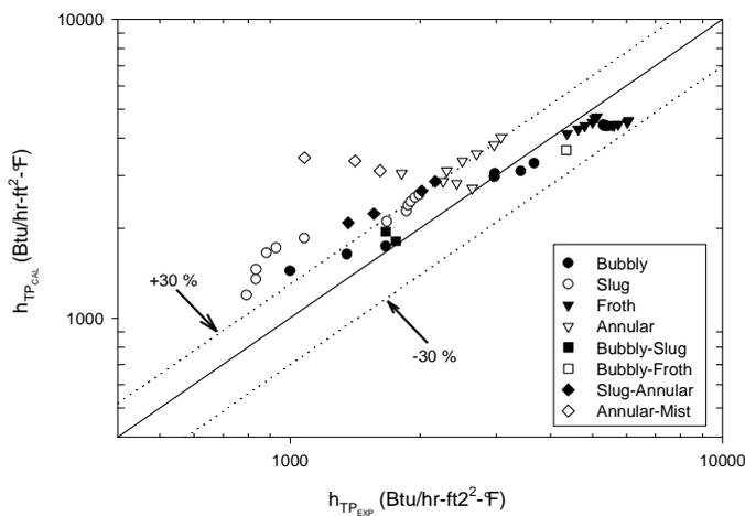
Figure 14. Comparison of Chu and Jones (1980) correlation with Aggour (1978) water-helium experimental data in a vertical pipe.
