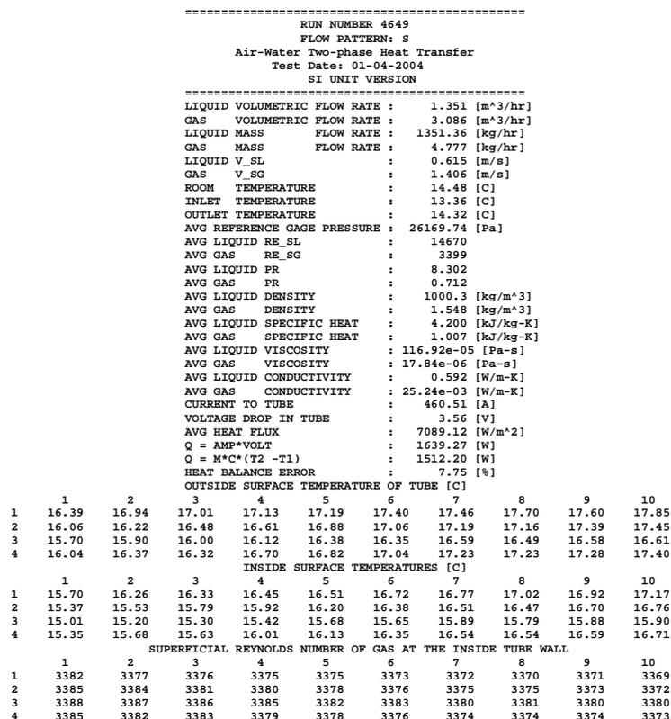
Figure 9. Data reduction program's output file for a test run.
