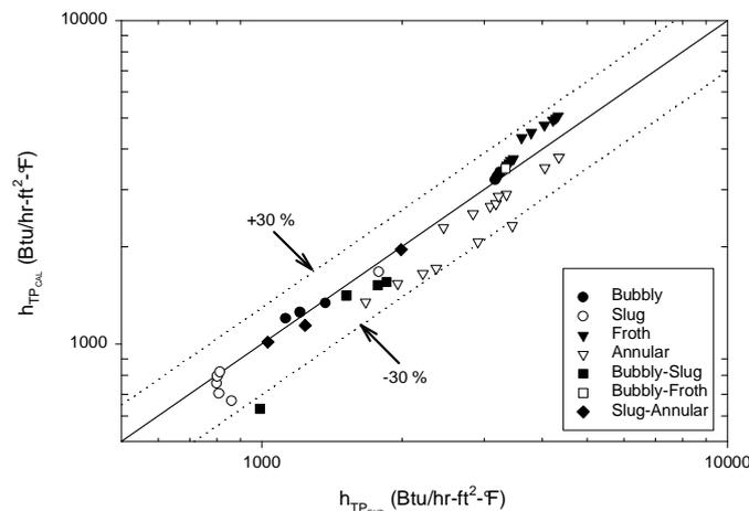
Figure 16. Comparison of Martin and Sims (1971) correlation with Aggour (1978) water-freon 12 experimental data in a vertical pipe.
