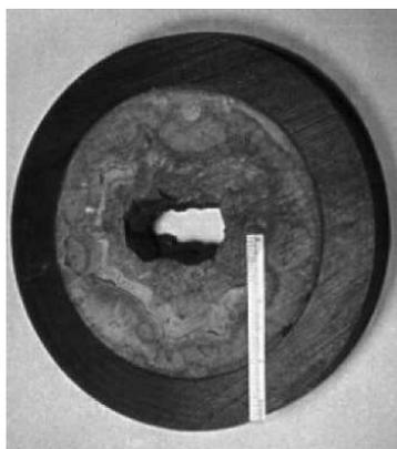
Figure 1. Wax deposition blockage in pipelines; adopted from Fogler (2004).
