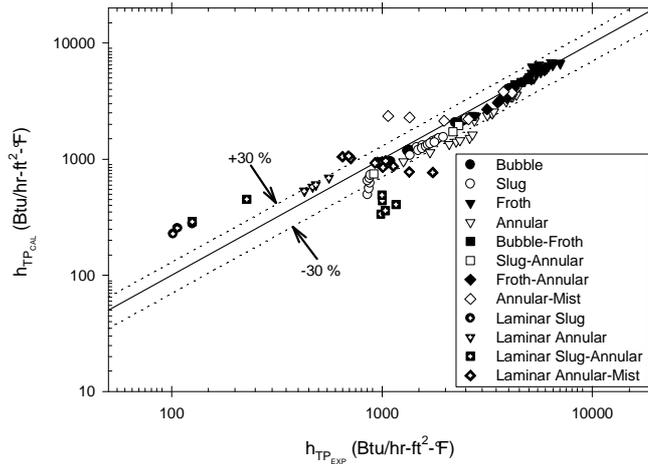
Figure 12. Comparison of Knott et al. (1959) correlation with Vijay (1978) air-water experimental data in a vertical pipe.
