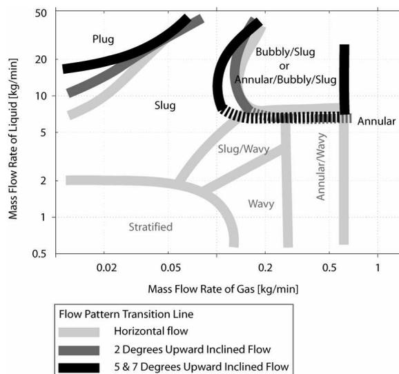
Figure 24. Change of flow pattern transition lines as pipe inclined upward from horizontal.
