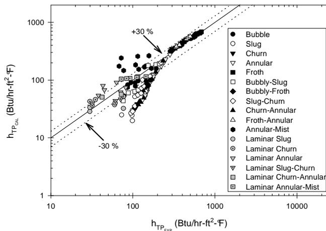
Figure 13. Comparison of Shah (1981) Correlation with Rezkallah (1987) Silicone-Air Experimental Data in a Vertical Pipe.
