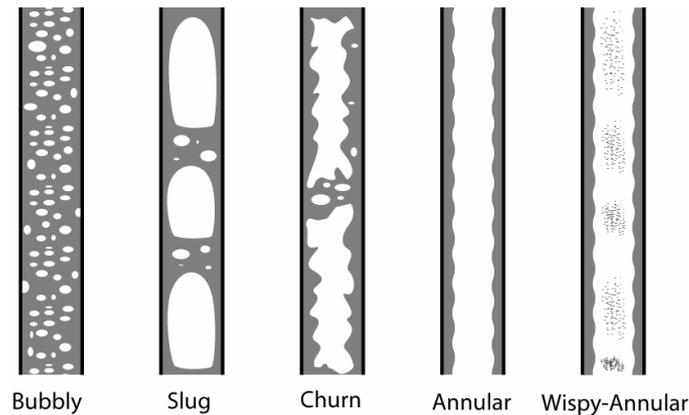
Figure 2. Flow patterns in vertical upward flow in a tube.
