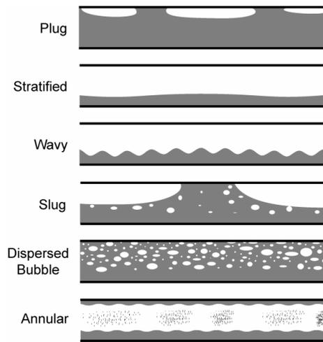
Figure 3. Flow patterns in horizontal and slightly upward inclined flow in a tube.
