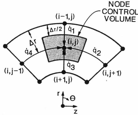
Figure 8. Finite-difference grid arrangement (Ghajar and Zurigat, 1991).
