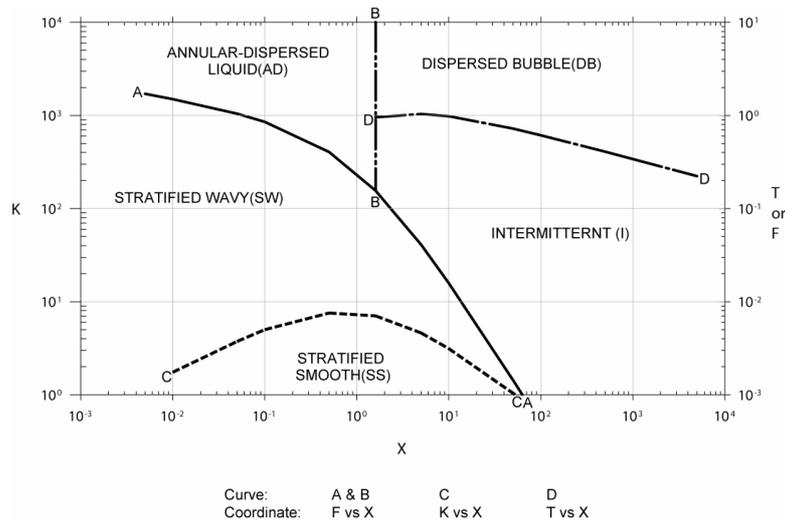
Figure 5. Taitel and Dukler (1976) map for horizontal flow.
