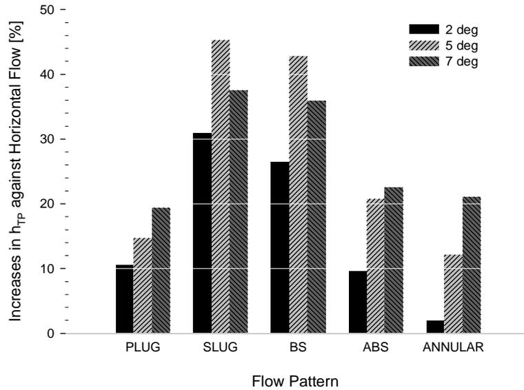
Figure 27. Increases of inclined flow  $h_{TP}$  against horizontal flow  $h_{TP}$ .
