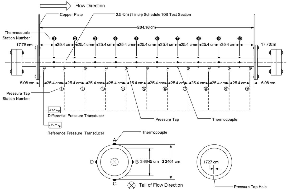
Figure 21. Test section.
