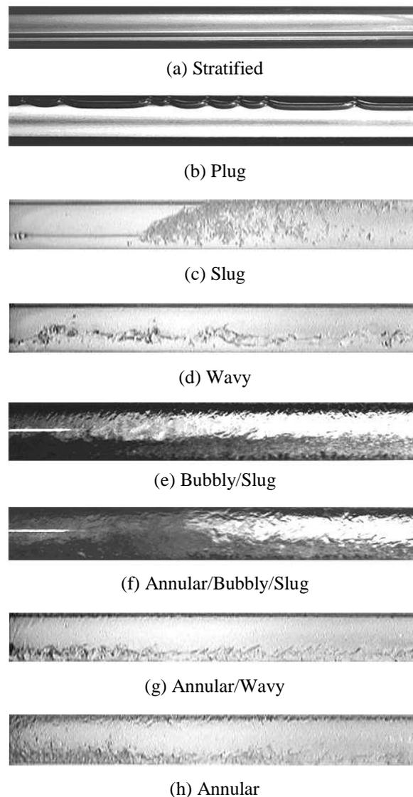
Figure 22. Photographs of representative flow patterns (horizontal flow and isothermal).
