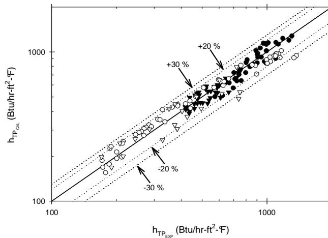
Figure 18. Comparison of the predictions by general correlation, eq. (62) with the experimental data for horizontal flow (150 data points).
