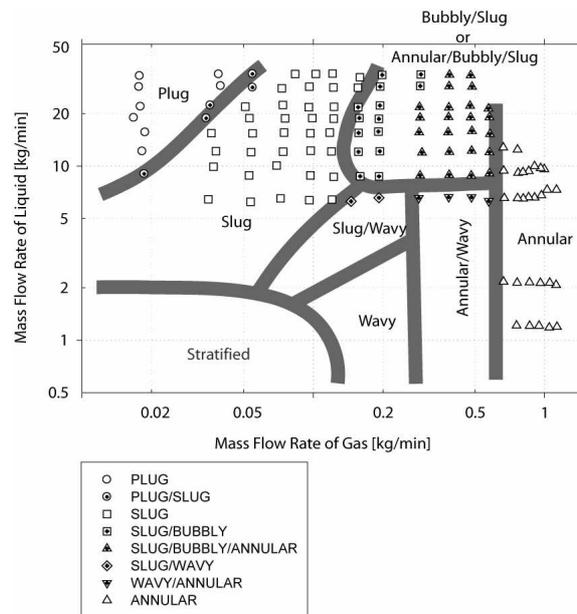
Figure 23. Flow map for horizontal flow.
