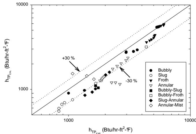
Figure 15. Comparison of Shah (1981) correlation with Aggour (1978) water-helium experimental data in a vertical pipe.
