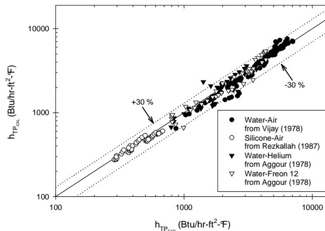
Figure 17. Comparison of the predictions by the general correlation, eq. (62) with the experimental data for vertical flow (255 data points).
