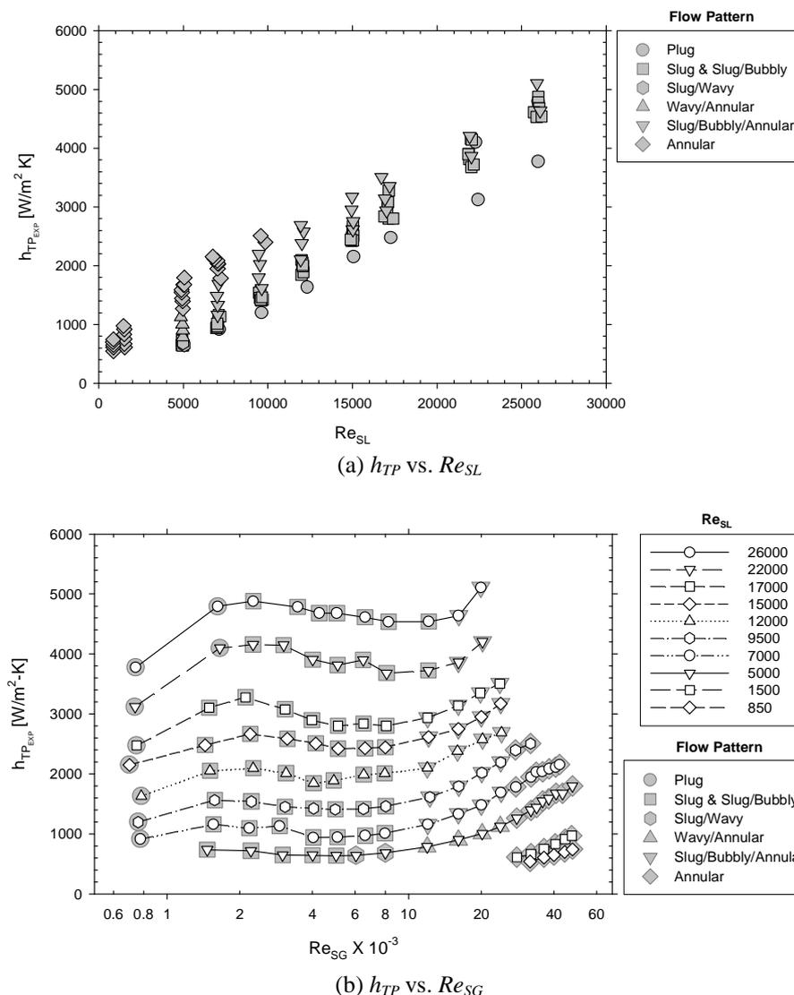
Figure 25. Variation of two-phase heat transfer coefficients with superficial liquid and gas Reynolds numbers in a horizontal flow.
