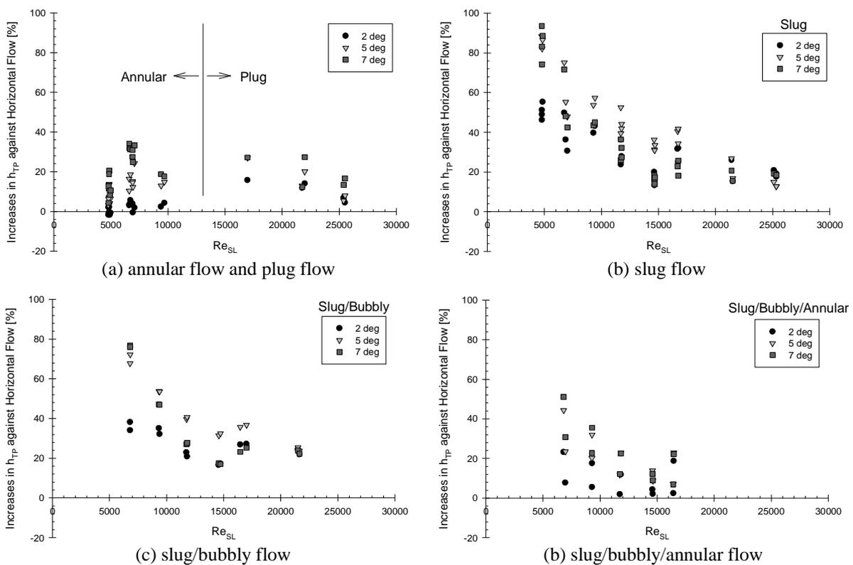
Figure 28. Increases of inclined flow  $h_{TP}$  against horizontal flow  $h_{TP}$  by flow pattern.
