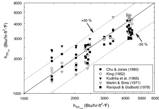
Figure 11. Comparison of selected correlations with King (1952) slug flow air-water experimental data in a horizontal pipe.
