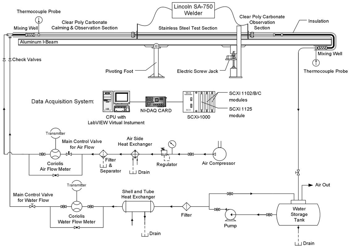
Figure 19. Schematic of experimental setup.
