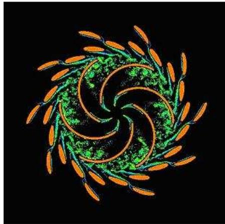
Figure 9. Instantaneous flow pattern in a pump-turbine during turbine-operation.
