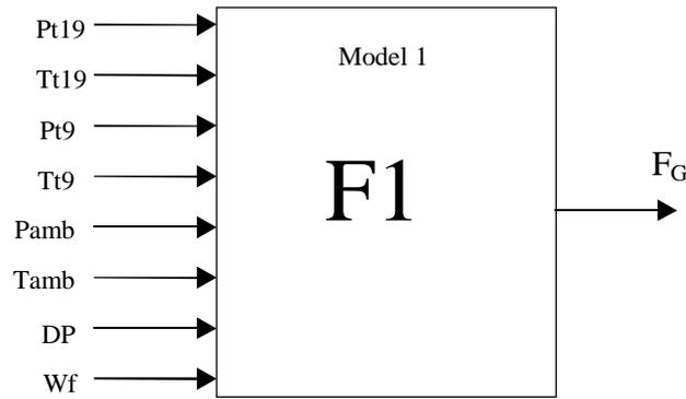
Figure 2 - Representation of a method for the determination of in-flight thrust - Method 1
