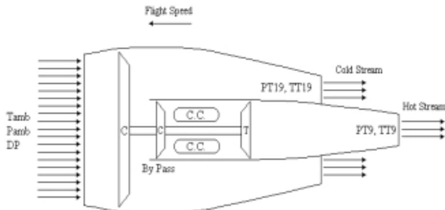
Figure 1 - Unmixed turbofan engine schematics
