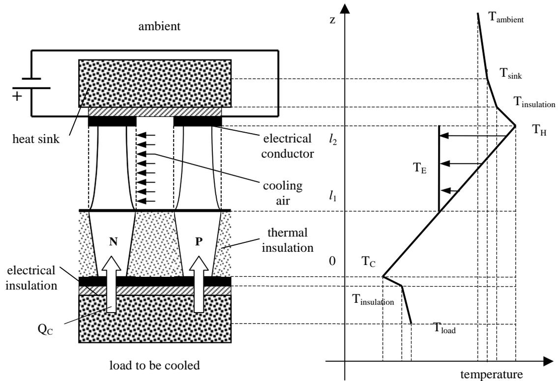
Figure 1 – Schematic view of a solid–state Peltier-effect cooling device with variable circular cross-sectional area arms.
