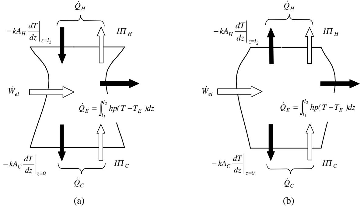
Figure 2 - The first law of thermodynamics for the concave (a) and convex (b) columnar arms of the Peltier-effect cooling device.
