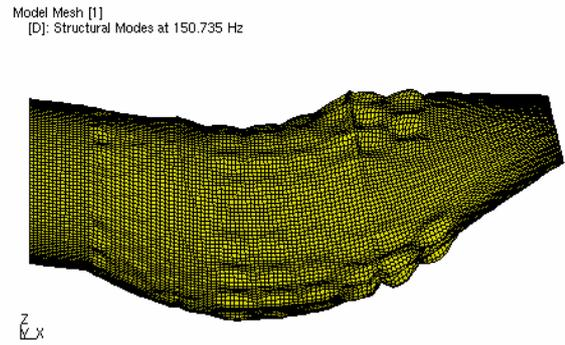
Figure 3b: Second structural bending mode
