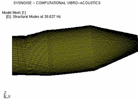
Figure 3a: First structural bending mode
