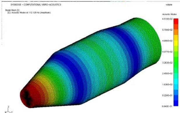
Figure 4b: Second acoustic longitudinal mode
