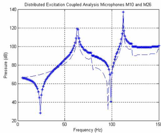
Figure 5: acoustic pressure spectra for uniform exterior pressure loading
