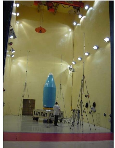
Figure 7b: Fairing and control microphones inside the 1,200 m<sup>3</sup> ARTF
