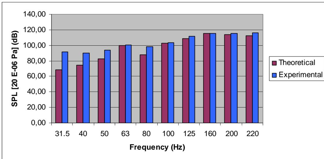
Figure 9: Low-frequency theoretical X experimental comparison
