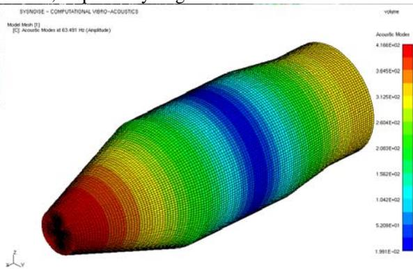
Figure 4a: First acoustic longitudinal mode
