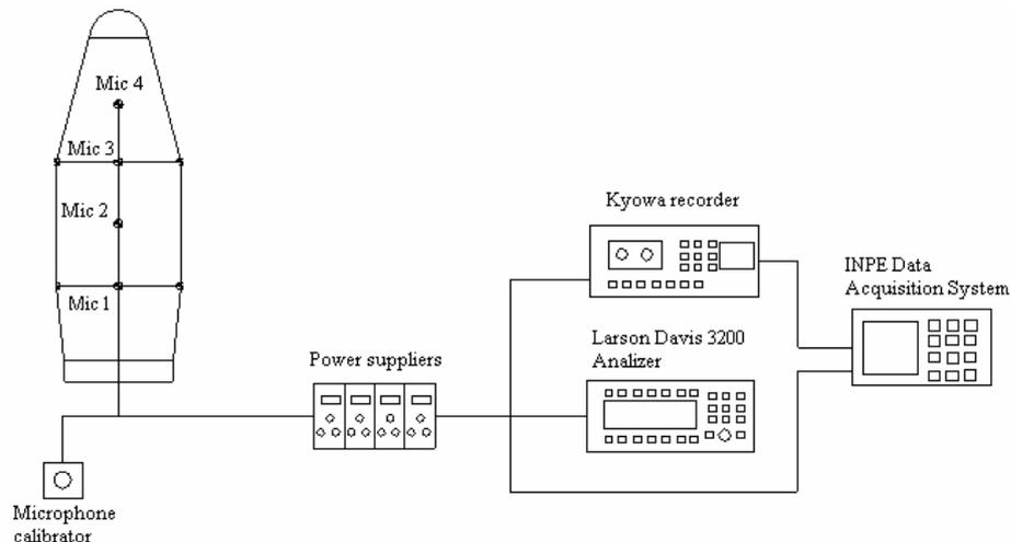
Figure 8: Data acquisition system and internal microphones location for the acoustic test
