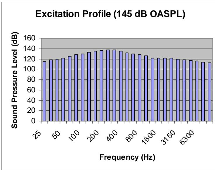
Figure 7a: VLS acoustic diffuse field for lift-off
