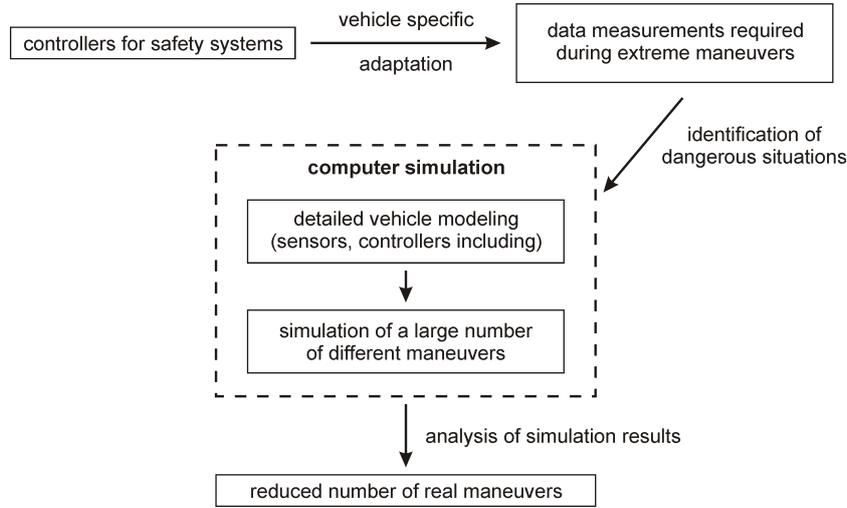
Figure 1 – Vehicle dynamic simulations to support the controller development.
