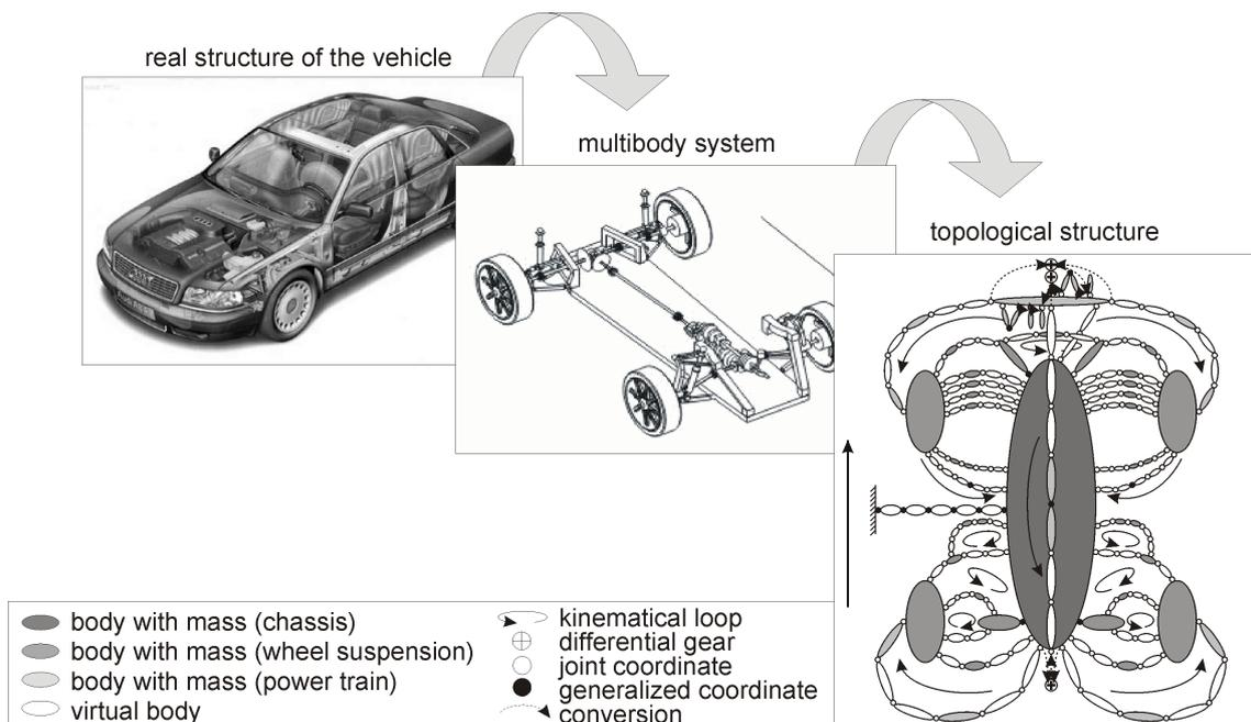
Figure 7 – Kinematic topology of an all-wheel driven upper class passenger car.
