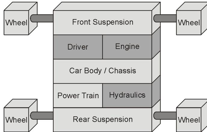
Figure 6 – Modular structure of a passenger car in FASIM\_C++.
