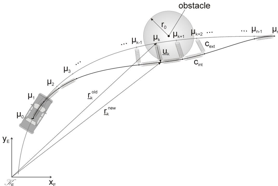
Figure 3 – Principle of the path planning with elastic bands.
