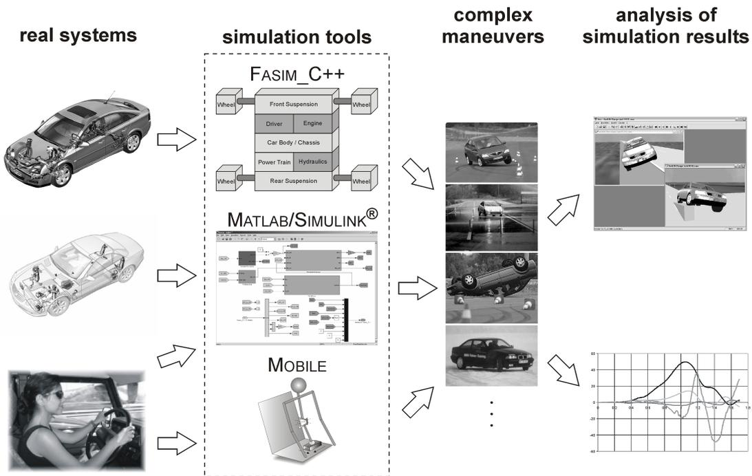
Figure 2 – Concept of the simulation environment for complex driving maneuvers.
