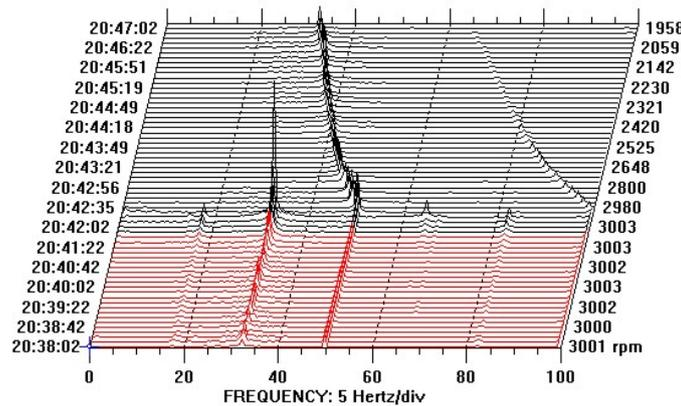
**Figure 4: Waterfall plot of the shaft vibrations measured at bearing #1 in occasion of a steam-whirl instability onset and during the subsequent coast-down caused by the machine trip.**
