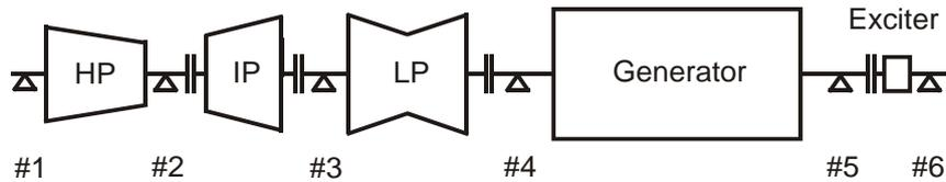
**Figure 1: Machine-train layout and bearing numbers.**
