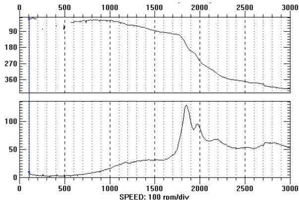
**Figure 2: Synchronous transient vibrations (1X) measured at bearing #1 of the HP turbine: passing through the first critical speed.**
