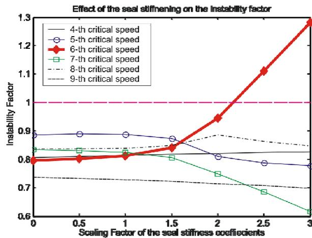
Figure 5: Instability factor versus exciting constant scaling factor
