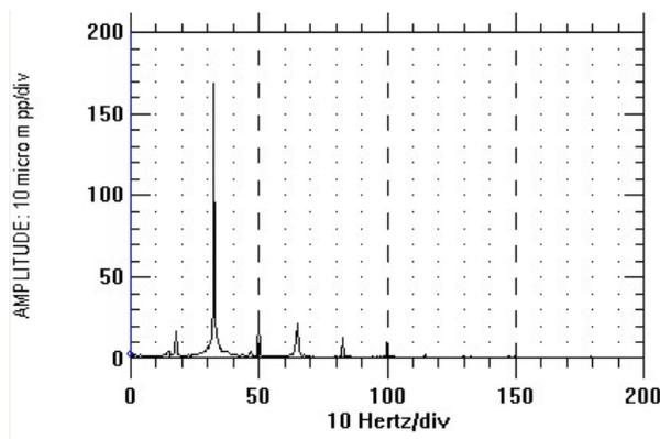
**Figure 3: Spectrum of the shaft vibrations measured at bearing #1 in operating condition before the onset of the instability.**
