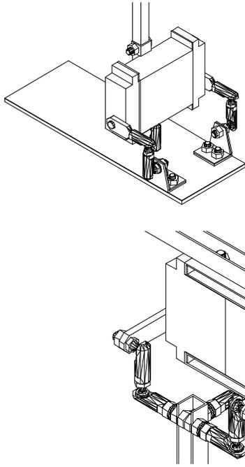
Figure 1: Ankle and Hip linkages
