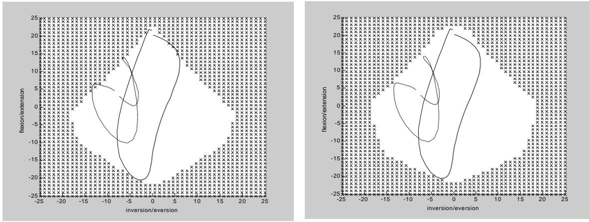
Figure 5: Workspace and gait trajectories for Solution 2 (left) and Solution 3 (right). The continuous line is the hip angular displacements in one gait cycle, and the dashed line represents ankle angular displacements.
