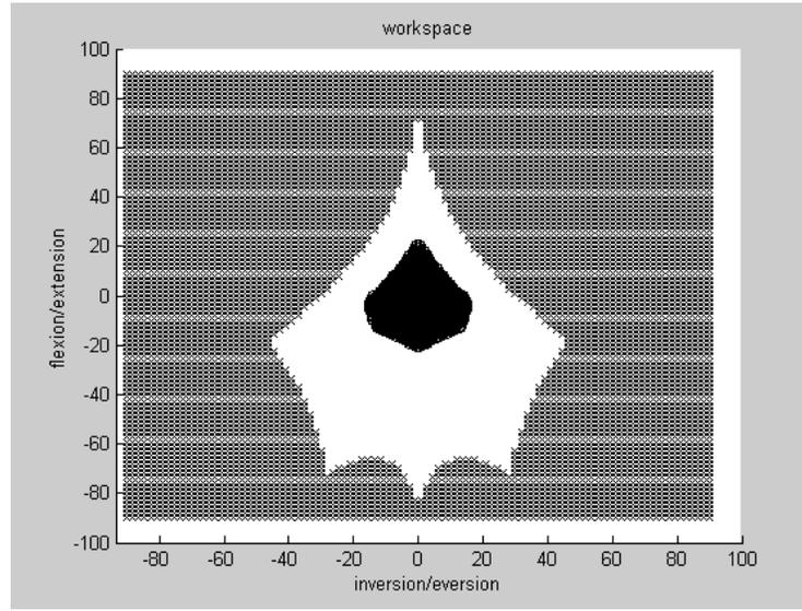
Figure 4: Workspace for a particular set of linkage dimensions. The lightest region corresponds to the real solutions of the linkage kinematic model, and the dark the workspace where the spherical joints are inside their angular displacement limits.
