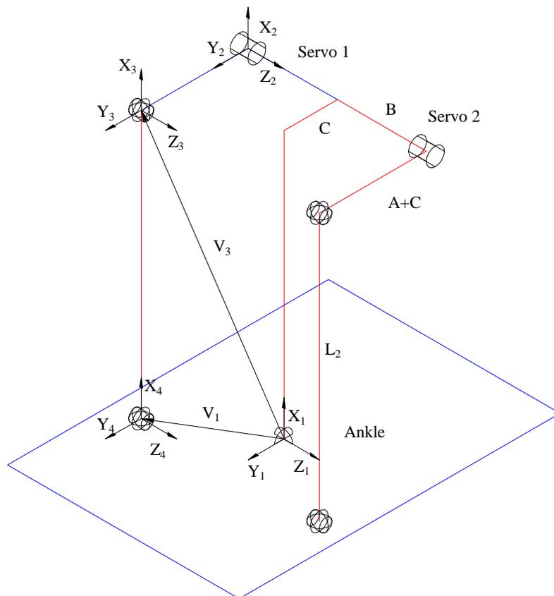
Figure 3: Kinematical model of the linkage used in robot's ankle.
